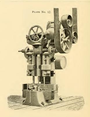
THREE-SPINDLE RAIL DRILLING MACHINE.
