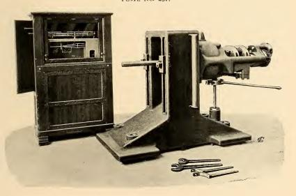
30,000-LB. DYNAMOMETER AND SCALE-CASE. FOR WEIGHING TRACTIVE FORCE OF LOCOMOTIVES. Centre of draw-bar adjustable from 28" above foundation to 46". these beams, 65 and 69, are rigidly united, the blow is absorbed by the total mass of these two beams. The hydraulic support is thus thoroughly protected, and these machines can be used regularly for breaking high steel specimens up to the full capacity of the machine without any risk of injury.
