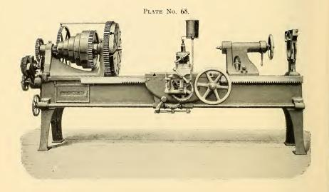
26" LATHE.—TRIPLE-GEARED, TURNING AND SCREW-CUTTING FEEDS.
