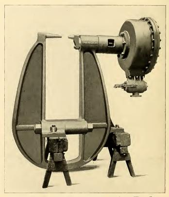
5-FT. STEAM RIVETING MACHINE—with Extra Wide Gap.
