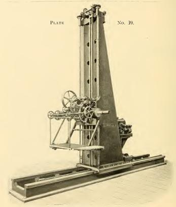
FLOOR-BORING MACHINE ON INDEPENDENT BED.
