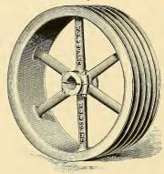
the best of their kind. The transmission wheels should be of *iron*, and have turned grooves of sizes and shapes that have been proved by long experience to be best for the purpose. They should be properly balanced, the various grooves should be so accurately turned to the same pitch diameter, that all of the ropes, or the various wraps of the same rope, may travel at the same velocity, and they should be so fitted and attached to the shaft that the grooves will "run true" and without vibration.
