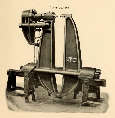
HYDRAULIC RIVETING MACHINE. 7 FEET GAP, 100 TONS PRESSURE ON DIES.
