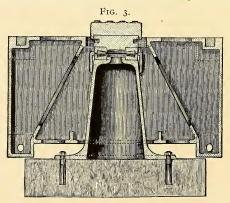
wheels that bear on the circular track and take the tip of the table when the load is not balanced. The pivot centre itself consists first of a conical post with a broad base, for bolting securely to a large capstone upon a suitable foundation.
