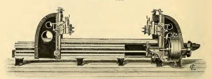
36" ROD PLANER-TO PLANE RODS FROM 3 FEET TO 12 FEET LONG.
