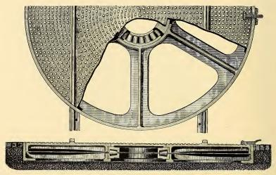
put it in motion from a state of rest. All turn-tables that we build are erected in our works, carefully fitted and properly marked for assembling, so that our customers will have no fitting to do except trimming the wooden packing so as to bring the table to the proper level. This is a simple matter.
