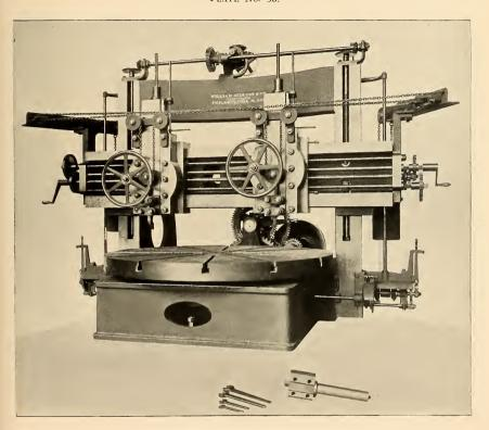
7-FOOT BORING AND TURNING MILL-WITH TWO SADDLES.
