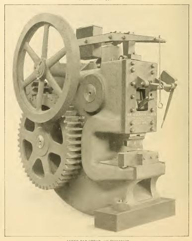
LEVER BAR SHEAR—10" OVERREACH. For cutting steel bars up to 12'' by 29''. Patent toggle-joint stop motion. Fast and loose pulleys, 36'' diameter, 7'' face, 240 revolutions per minute. Shear blades may be set at right angles to position shown for cutting long bars. Counterbalanced slide.
