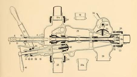
When it is especially desired to use supply water at a high temperature, a new form of this injector (Class K.) can be supplied, for which the limiting temperature is 145 degrees at 120 pounds of steam, and 140 degrees at 180 pounds pressure. The capacity of these injectors is given in the following table, which is based upon recent improvements that have largely increased the delivery at 180 and 200 pounds steam pressure.
