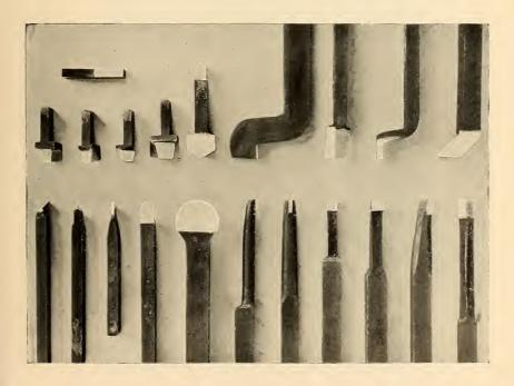
EXAMPLES OF MISCELLANEOUS THREAD, BORING, SLOTTING, AND OTHER TOOLS OF DIFFICULT SHAPES,
