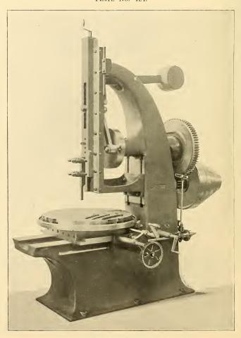
From face of tool to frame, 21". Stroke adjustable from o" to 12". Uniform cutting speed and quick return. Table, 28" diameter, with rotary, transverse and longitudinal motions. Variable self-feed occurring at top of stroke, and all crank handles in a convenient position. Table has water-trough. Transverse and longitudinal travel of table, 20". Floor to top of table, 32%". Extreme height from top of table to underside of frame, 135".
