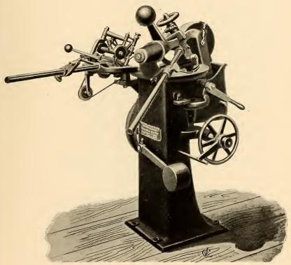
FRONT VIEW OF PATENT DRILL-GRINDING MACHINE.
