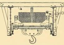
SECTION THROUGH BRIDGE WITH TROLLEY IN POSITION,
