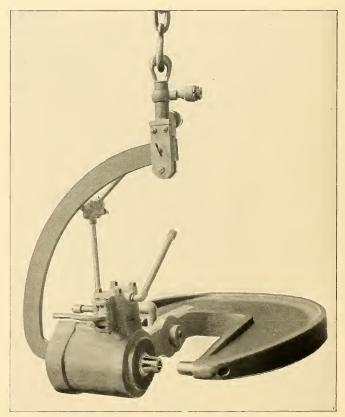
DIRECT-ACTING PORTABLE HYDRAULIC RIVETER.
