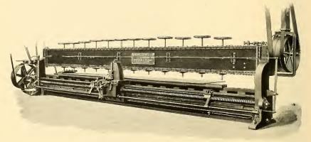
PLATE-PLANING MACHINE—WITH END-PLANING ATTACHMENT FOR PLATES 22 FT. LONG, 5 FT. WIDE, AND 2" THICK, AT ONE SETTING.
