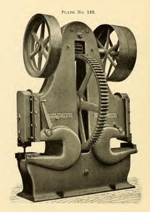
PUNCHING AND SHEARING MACHINE COMBINED.
