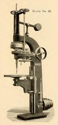
36" VERTICAL DRILLING MACHINE—WITH CIRCULAR TABLE.
