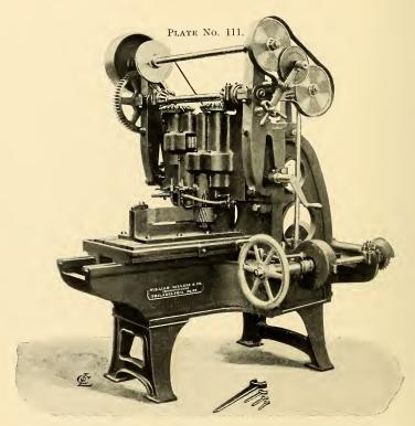
TWO-SPINDLE VERTICAL MILLING MACHINE—FOR TEST SPECIMENS.
