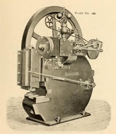
BAR SHEAR-WITH PUNCHING ATTACHMENT.
