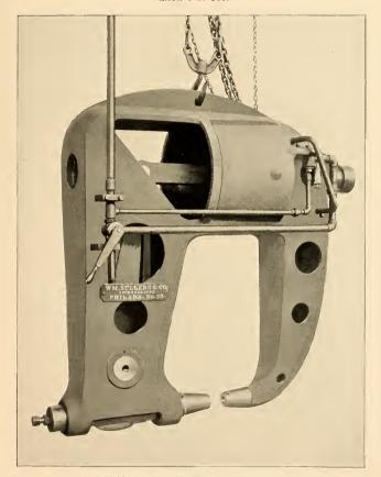
PORTABLE PNEUMATIC RIVETER.
