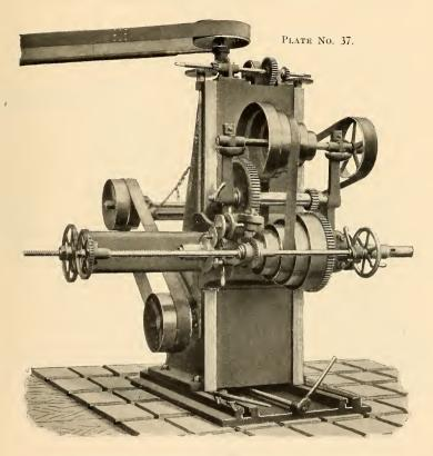
FLOOR-BORING MACHINE—DRIVEN BY BELT AND SWING FRAME.
