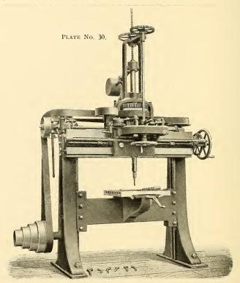
TRAVERSE-DRILL WITH COTTER DRILLING ATTACHMENT. FOR KEYSEATS, SLOTS, ETC.
