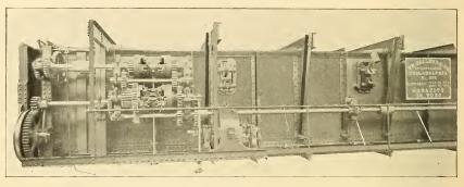
50-TON TRAVELLING CRANE.—SINGLE MOTOR TYPE.
