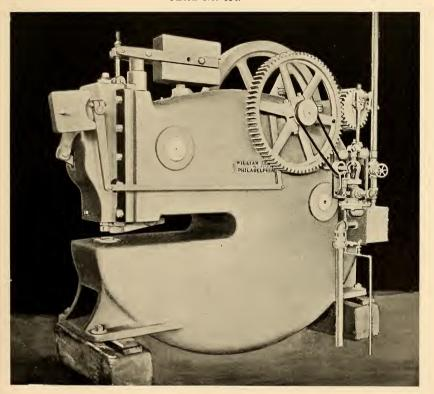
36" LEVER PUNCHING MACHINE—with 8" x 8" Engine.
