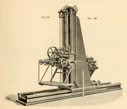
FLOOR-BORING MACHINE WITH MILLING AND BORING FEEDS.
