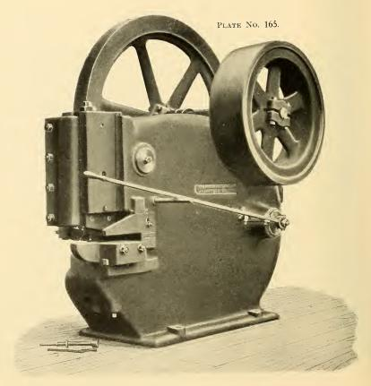
BAR SHEAR-with Punching Attachment.
