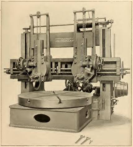
7-FOOT BORING AND TURNING MACHINE—For STEEL RAILWAY TIKES, ETC.
