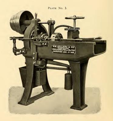
1½" PATENT BOLT AND NUT-SCREWING MACHINE.
