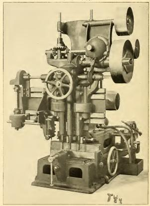
THREE-SPINDLE DRILLING MACHINE. WITH COMPOUND BASE FOR GIRDER RAILS.
