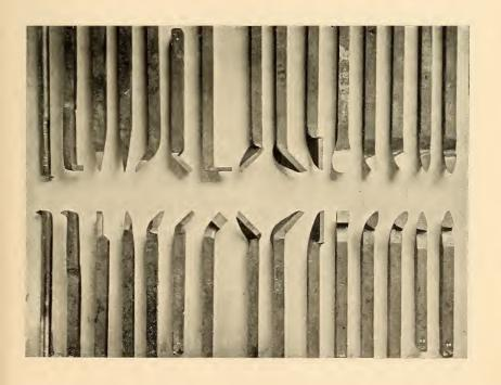
EXAMPLES OF LATHE TOOLS FINISHED TO SHAPE BY THE TOOL-GRINDING AND SHAPING MACHINE.
