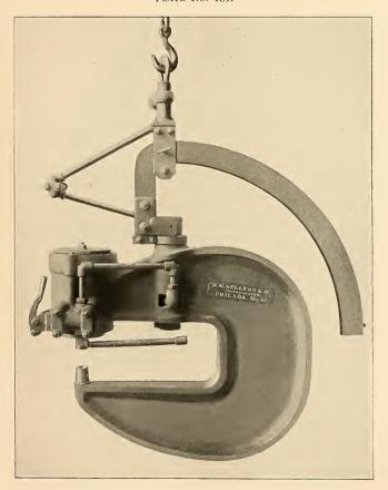
DIRECT-ACTING PORTABLE HYDRAULIC RIVETER.
