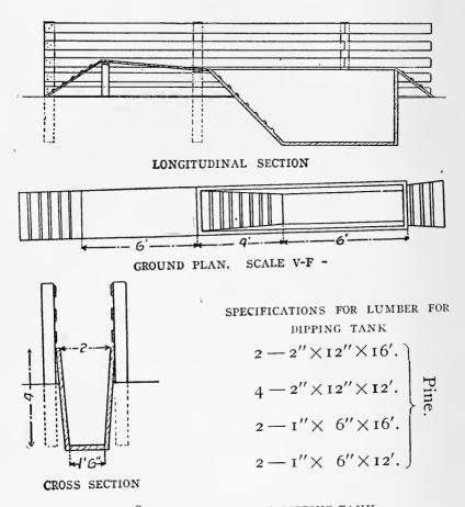
FIG. 18—PLAN FOR GOODELL DIPPING TANK
