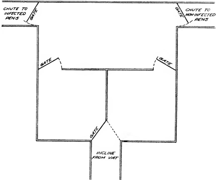
FIG. 1.—Plan of draining pen for cattle after dipping.
