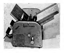
pletely portable, the Auto-Fold will handle stock up to 9½inches wide by 14-inches long. The machine can be easily set for single, double, standard, accordion, French, and many other folds by following the folding chart permanently inscribed on the side of the machine. Martin-Yale
