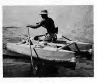
float construction affords unusual stability and freedom from tipping and rocking. It is convenient to launch and beach as one man can stand between the floats, pick up the craft, and easily carry it in or out of the water. Available in two sizes: the standard and the larger crew-size model. Selleck Watercycle Company, Inc., Catamaran Division, Boca Raton, Florida.
