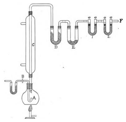
where the steam condenses, then through the two drying tubes "D" and "E," containing calcium chloride and sulphuric acid, respectively, which remove the last traces of the water vapor. Finally, the carbon dioxide remaining, passes into the two sodalime tubes "1" and "2" where it is absorbed.
