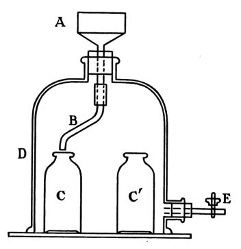
has been exhausted. C,C' are 4 oz. wide-mouth bottles. By rotating A, B may be made to deliver into the different bottles successively. The apparatus used by the Chairman will hold five bottles.
