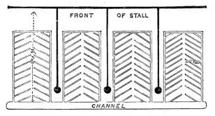
Stalls with grooves in floors inclining backwards and outwards to side grooves.
