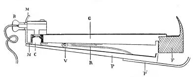
Fig. 179.—Longitudinal and median section of the *chaussure exploratrice*. (Same letters as in Fig. 178, except *F*, which represents the section of the shoe at the toe.)
