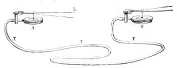
Fig. 173.—Two drums with a lever and tubing to carry the compressed air. (Marey.)
