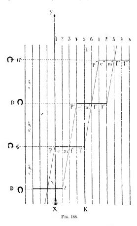
Such is the principle of the ingenious method of M. Lenoble du Teil. It has the advantage of recording all the data relative to the *duration* and the *space passed over* which the registering apparatus or chrono-photography can collect from a given gait. When the diagram is once constructed, all desirable information relative to a complete analysis of the phenomena can be obtained at a glance in a concise form and compared the one with the other, which is not to be overlooked.
