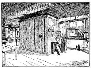
ATWATER'S RESPIRATION CALORIMETER. A Man Lives in the "Box" for Days and the Actual Heat and Energy Obtained from the Food Consumed is Determined. (See page 52.)
