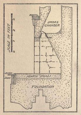
A cross-section showing the construction of a large stone fireplace with slightly arched opening
