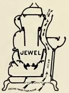
Sectional View Showing the Plan or the lewel Double Heating Flue
