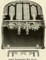
The grate consists of a series of triangular bars, which when turned cuts the ashes and clinkers from the fire, without dropping unburned fuel into the ash pit. No bolts or nuts are employed and the bars can be removed by lifting the cast yoke from place and removing the iron cogwheels which hold them in place. (See illustration.) So simple is the construction that a bar can be taken out or replaced while the fire is burning.
