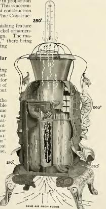
In Shape for infree reasons: First, because it eliminates dead surfaces; second, because it gives the great-res cold air form foor, heats it while passing upward and expels it heated to a temperature of over 250 degrees. The above is from careful test while stove was moderately burning.
