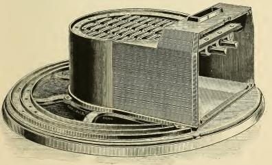
The above cut illustrates the triangular revolving grates used in all the STAMFORD FURNACES. They are strong and well fitted, and are so constructed that, should necessity for repairing ever arise, they can be easily removed by simply loosening two bolts immediately in front, without disturbing any other part of the furnace.
