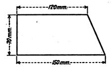
This tin-foil wrapping should be made of foil weighing 80 to 100 g. per square meter. The charge is wrapped in such a manner that a cartridge of the exact size as the diameter of the hole is formed. After the cartridge is completed, an electrically detonating charge of 2 g. is inserted in the center of it, and the whole is
