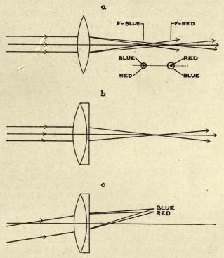
FIG. 6.—(a) Chromatic aberration in a single collective lens. (b) Doublet corrected for axial chromatism.
