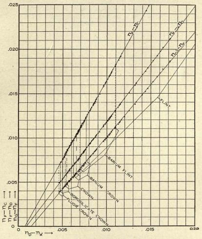
FIG. 16.—In this figure the partial dispersions,  $n_F - n_D$  and  $n_G' - n_F$  of all silicate optical glasses listed by Parra-Mantois and by Schott, are plotted as ordinates against the partial dispersion  $n_D - n_A'$  as abscissæ. The result in each case is a straight line.
