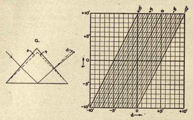
FIG. 88.—In this diagram are given the deviations of the emergent ray, from the prescribed path, after transmission through a right-angle prism of slightly incorrect interfacial angles as indicated in fig. 88a.
