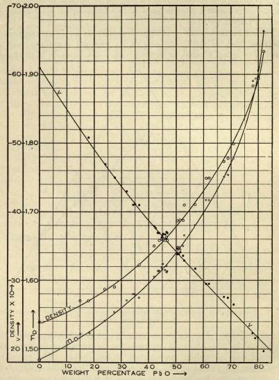
FIG. 20.—In this diagram there are shown the changes in the density and the optical constants (refractive index,  $n_{\rm D}$ , and  $\nu$ ) with changes in lead oxide (PbO) in the flint series of glasses.
