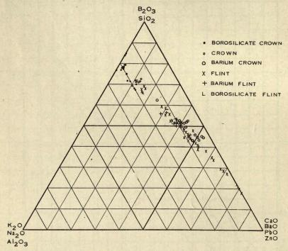
FIG. 22.—Triaxial diagram showing the weight-percentage compositions of the ordinary crowns, boroilicate crowns, barium crowns, flints, barium flints, and borosilicate flints of Table 4.
