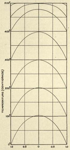
F10.55.—Curves representing the temperature distribution in a sphere of glass of unit radius cooling at a linear rate from 500° C. to 0° C. The zero abscissa represents the center of the sphere.
