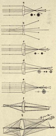
(positive) lens. (b) Spherical aberration in a single dispersive (negative) lens. (c) Doublet corrected for spherical aberration. (d) Spherical overcorrection in a doublet. (e) Spherical zones in a doublet corrected for spherical aberration. (f) Coma in a lens. Lack of fulfillment of sine condition. (g) Astigmatism in a lens.
