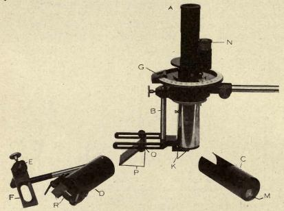
FIG. 71.—The Koenig-Martens hand photometer with special attachments for use in measuring light transmission of optical glass plates and optical instruments. A, the photometer; N, a scale-reading lens; B, an attachment supporting the two reflecting prisms, K and P; C, a tube with eccentrically mounted lens M for use in measuring light transmission in optical instruments; D and E, attachments used in measuring the amount of normally incidentlight reflected from a polished glass surface.
