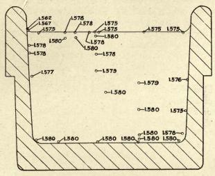
FIG. 41.—Diagram illustrating changes in refractive index, n<sub>D</sub>, at different parts of a pot of light flint glass after two hand-stirring periods of 15 minutes each Pot No. 472, Bausch & Lomb Optical Co.
