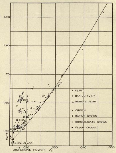
FIG. 14.—In this diagram the dispersive powers of a series of optical glasses are plotted against their refractive indices,  $n_p$ .
