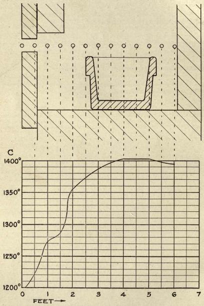
F16.27.-Cross section of melting furnace, showing points at which temperature measurements were made with the water-cooled rod of fig. 26. Below is the corresponding distance-temperature curve.
