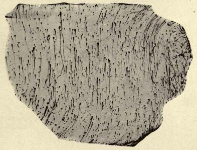
FIG. 39 .-- Photograph of sand grains in process of solution in a small melt of optical glass.
