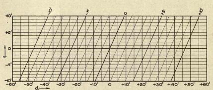
FIG. 89.—Constant deviation method. In this figure the deflections are shown of the emergent ray from the prescribed path, after transmission through a prism of slightly incorrect interfacial prism angles, as indicated in fig. 89a.
