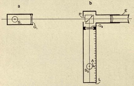
FIG. 69.—Apparatus for the measurement of the light transmission in optical glass plates.  $S_1$  and  $S_2$  are electric lamp bulbs;  $G_1$  and  $G_2$ , thin plates of milk glass;  $P_1$ , a Lummer-Brodhun photometer prism; L, graduated scale; A, position indicator for the lamp  $S_2$ ;  $E_1$ , eyepiece. Designed and manufactured by Keuffel and Esser.
