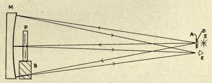
FIG. 61.—Concave mirror test for the inspection of striae in plates of optical glass. S is source of light; D, ground glass diffusing disk; A, pinhole aperture; M, a concave mirror; P, plane parallel plate of glass: E, the observer's eye.
