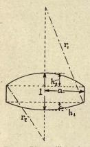
FIG. 74.—Diagram illustrating the several elements necessary to compute the volume of a lens. L is the thickness of the lens; a, the semidiameter;  $r_1$  and  $r_2$ , the radii of curvature;  $h_1$  and  $h_2$ , the height of the spherical segments.
