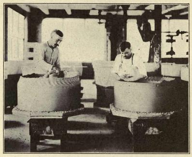
FIG. 24.—Clay pots in the making by the hand "building-up" process. (Photograph by J. Harper Snapp at the plant of the Bausch & Lomb Optical Co.)
