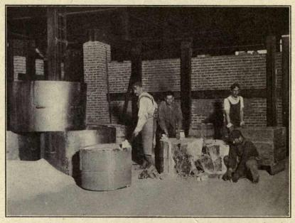
FIG. 43.—Breaking apart pots of optical glass. Note the sheet-iron insulating cap on left, also storage box for pot of optical glass on right of photograph. (Photograph by J. Harper Snapp at plant of Bausch & Lomb Optical Co.)
