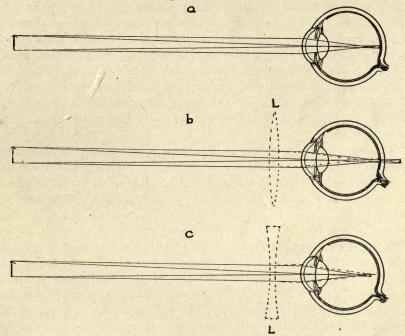
FIG. 2.—Diagrams illustrating action of eyelens in forming image of distant object on the retina. Fig. 2a shows action of a normal eye in which the image is focused on the retina itself. In fig. 2b the image plane is located back of the retina (far-sighted eye), while in fig. 2c the image plane is in front of the retina. The dotted lines in fig. 2b and 2c illustrate the action of spectacle lenses in increasing (fig. 2b) or decreasing (fig. 2c) the convergence of the incident rays.
