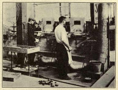
FIG. 75.—The pressing of small lenses and prisms. (Photograph by J. Harper Snapp at plant of Bausch & Lomb Optical Co.)
