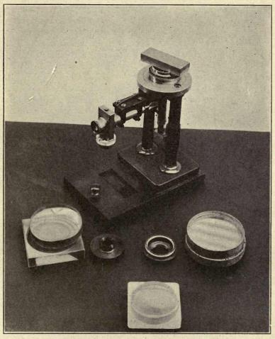
FIG. 81.—Spherometer and test-plates for measuring radii of curvature of lenses. The test plates show the Newton color fringes. (Frankford Arsenal.)
