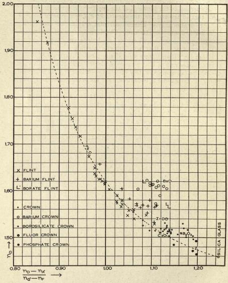
FIG. 15.—In this figure the ratio  $(n_{\rm D}-n_{\rm A}')/(n_{\rm G}'-n_{\rm F})$ , which expresses in effect the length of the red end of the spectrum to that of the blue end, is plotted against the refractive index  $n_{\rm D}$  for a series of different types of silicate optical glasses.
