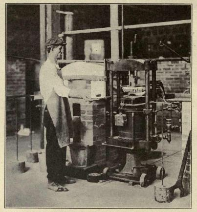
FIG. 53.—Block of glass in moldand ready to be pressed into plate by plunger of hydraulic press. (Photograph by J. Harper Snapp at plant of Bausch & Lomb Optical Co.)
