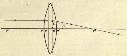
FIG. 4.—Diagram illustrating the principal Gauss points H and H' (planes), and the principal foci, F and F', of a lens for paraxial rays.
