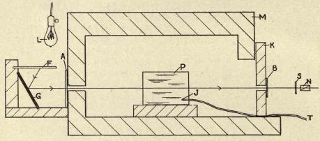
FIG. 54.—Simple arrangement adopted for the study of strain-temperature-time relations in optical glass. L is an electric bulb; F, a plate of frosted glass; G, a piece of opaque glass placed at the polarization reflecting angle; A, a piece of thin glass; M, the gas-heated annealing oven; P, the glass plate under test; T, the thermoelement; B, a thin glass window; S, a sensitive-tint plate: N, the analyzer.
