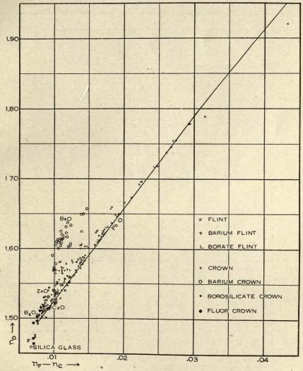
FIG. 13.—In this figure the mean dispersions,  $n_F - n_c$ , of a series of different types of silicate optical glasses are plotted against the refractive indices,  $n_p$ . The points of projection for the ordinary crowns and the ordinary fints fall on a practically straight line, as indicated in the diagram.
