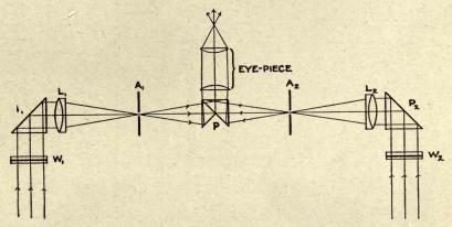
FIG. 70.—Photometer with neutral tint wedges for the measurement of the light transmission in optical glass plates.  $W_1$  and  $W_2$  are graduated neutral tint wedges;  $P_1$ ,  $P_2$ , reflecting prisms;  $L_1$ ,  $L_2$  objective, lenses; A1, A2, removable stops; P, photometer prism.
