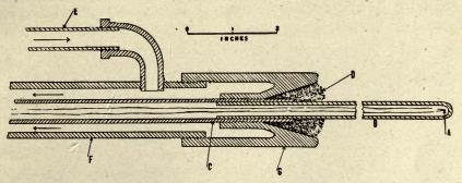
Fig. 26.—Sectional view of end of water-cooled temperature-measuring device. A is the hot junction of platinum-rhodium thermoelement; B, a refractory porcelain tube; C, inner iron pipe; D, asbestos packing; E and F, iron pipes of water-cooling system; G, specially turned iron terminus of water-cooling system.
