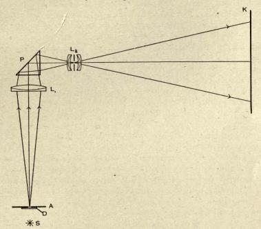
FIG. 87.—Projection method for prism inspection. S is the source of light; D, ground-glass diffusing disk A, pinhole aperture; L<sub>1</sub>, achromatic doublet; P, prism under test; L<sub>2</sub>, projection lens; K, projection screen.
