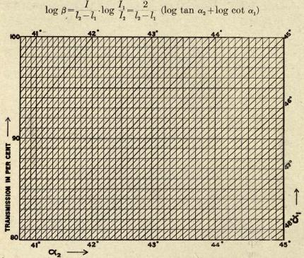
FIG. 73.—Graphical solution of the equation  $I = \tan^2 \alpha_2 \cot^2 \alpha_1$  used in connection with the polarization photometer. The abscissae represent the angles  $\alpha_2$ ; the sloping lines, the angles  $\alpha_1$ ; and the ordinates, the percentage light transmission, I.
