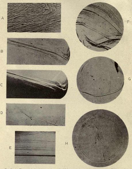
FIG. 7.—(a) Heavy striæ in a plate of glass. (b) Ribbon striæ (central illumination). (c) Ribbon striæ (oblique illumination). (d) Cord in a plate of glass; stone with striæ streamers near top of plate.
