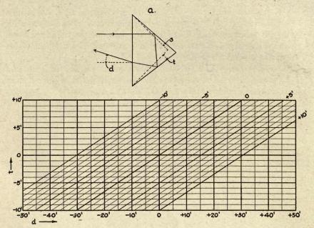
FIG. 91.—Autocollimation method. A graphical representation is given in this diagram of the deviations of the emergent ray from the prescribed path, after transmission through a prism of slightly incorrect interfacial angles, as indicated in fig. 91a.
