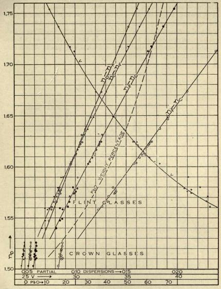
FIG.21.—In this diagram the changes in the partial dispersions,  $n_F - n_C$ ;  $n_D - n_A'$ ;  $n_F - n_D$ ;  $n_C - n_F$ , in the  $\nu$ -values and in the lead oxide (PbO) content with changes in refractive index,  $n_D$ , are shown for the flint series of glasses. The ranges of partial dispersions in the ordinary crown glasses with changes in the refractive index,  $n_D$ , are also illustrated.
