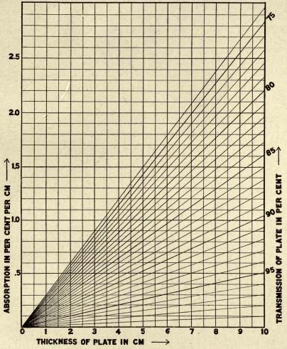
FIG. 68.—Graphical solution of the equation for light- transmission of plane-parallel plates. The abscissae represent the thickness of the plate in centimeters; the radiating lines, the percentage transmission of the glass plate; the ordinates, the absorption in per cent per centimeter glass-path.
