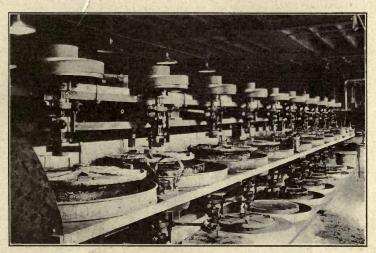
FIG. 57.—Grinding (lower row) and polishing (upper row) disks for plates of optical glass. (Photograph by J. Harper Snapp at the Hamburg plant of Spencer Lens Co.)
