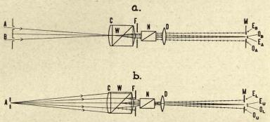
FIG. 72.—Optical arrangements of Koenig-Martens photometer. In fig. 72a the paths of the rays from the two apertures A, B, are shown; in fig. 72b the paths of the rays when only one aperture, A, is employed.
