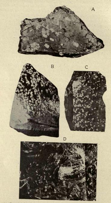
FIG. 9.—(a) "Stones" (spherulites of wollastonite) in glass; note also "joint" cracks developed on rapid cooling of the plate of glass. (b) Crystallization bodies in optical glass. (c) Spherulites of cristobalite on surface of barium crown melt. (d) Crystals of barium disilicate in barium crown glass.
