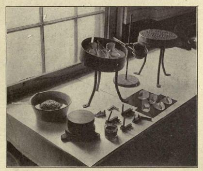
FIG. 79.—Prisms in process of blocking with plaster of paris for polishing. On the right there is a block of prisms ready for polishing. (Frankford Arsenal.)
