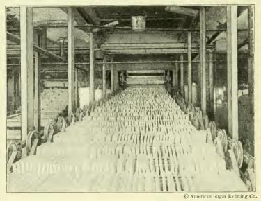
Fig. 51. Sugar on moving drying pans in a Jersey City sugar refinery
