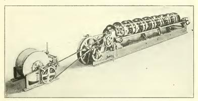
Fig. 36. A machine which twists the wires into strands
