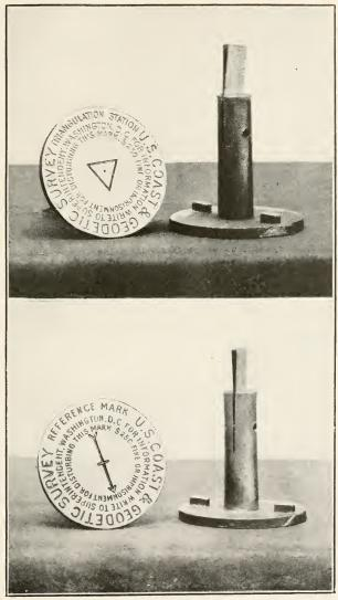
STANDARD STATION AND REFERENCE MARKS USED IN MARKING TRIANGULATION STATIONS.
