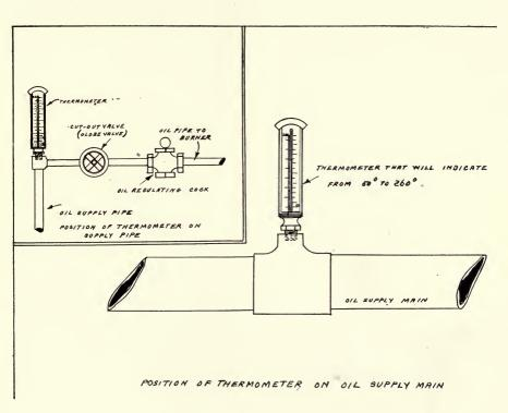
Fig. 1. Above cut illustrates manner of placing thermometers on main oil supply lines or on oil supply pipe to burner.
