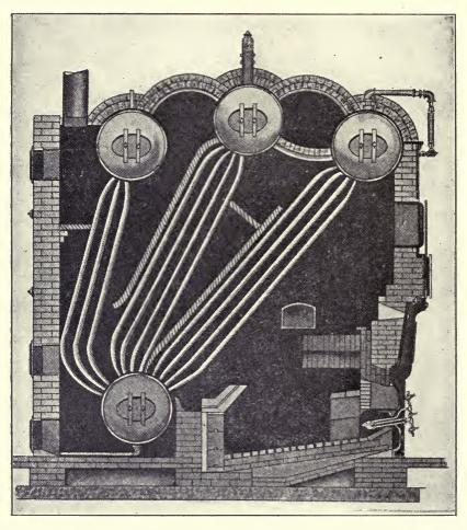
Fig. 6. Stirling Boiler Equipment.
