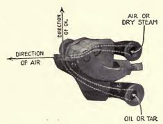
Fig. 1. High Pressure Oil Burner.
