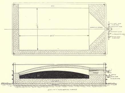
Plate Heating Furnace, charging space 18 ft. x 30 ft.
