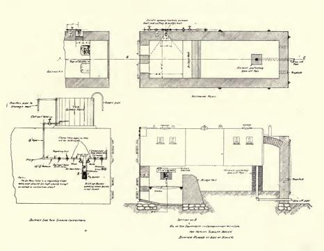
Fig. 2. Boiler equipped for the use of oil or tar to aid coal or breeze fire in carrying peak loads.
