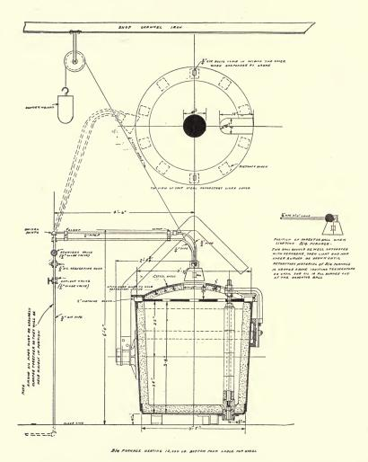
A 10,000 lbs. bottom pour ladle in steel foundry heated by a furnace which can be swung up and out of the way as soon as the ladle has been brought to the temperature required. The cover is then removed and the ladle placed in position to receive the charge.
