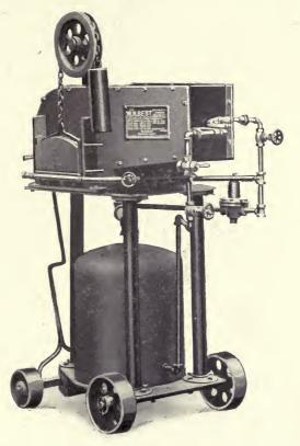
A self-contained portable outfit with 20 gallon oil tank, which can readily be moved around from place to place and which is used for heating 8,000 ¾-in. x 3-in. rivets in ten hours, as well as for forging, tool dressing, etc. Very convenient for small work in shops not equipped with the regular oil system as well as for work where portable outfit is necessary.
