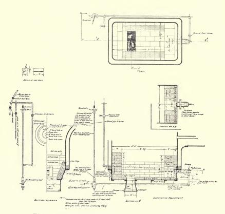
Fig. 2. Most modern type of locomotive equipment.
