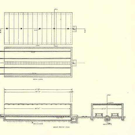
Fig. 1. Oven 44 ft. long, 20 ft. wide and 12 ft. high in the clear operated with one burner.
