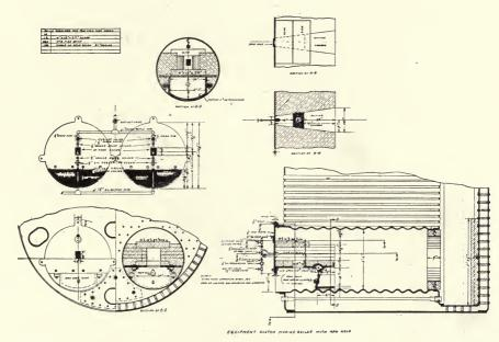
Fig. 5. Scotch Marine Boiler Equipment.
