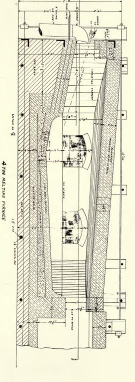
lurgists the ingots are stacked in their respective order, ready to be again melted in crucible furnaces. in order to dezinc same. In the latter case the metal is poured in ingots and after being analized by the metal-A 4 ton melting furnace used for various alloys and metals, or for melting large quantities of brass castings
