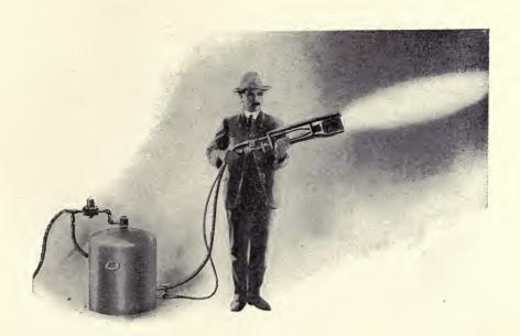
Hand Torches, made in various sizes, are very economical and efficient for all classes of light heating purposes, such as skin-drying moulds, lighting cupolas, heating tires, light brazing, burning paint off steel cars, etc.
