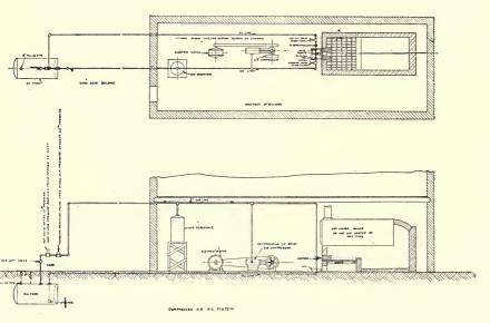
Fig. 4. Compressed Air System.
