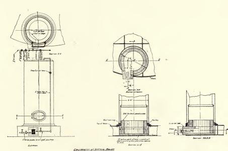
Fig. 12. Tangential Flame Equipment as applied to Vertical Boiler.
