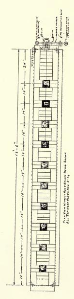
Fig. 1. A Multiple Ladle Heating Furnace used for heating ten ladles at a time and operated with only one burner.
