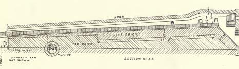
Fig. 1. A Continuous Billet Heating Furnace, 66 ft. long, 10 ft. wide, in which two rows of 12 in. square ingots 40 in. long are heated.
