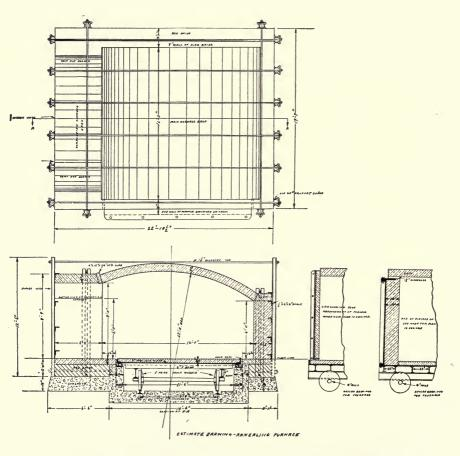
Overhead Oil-fired Car Annealing Furnace operated with only one burner.
