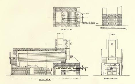
Equipment of Ore or Sand Roaster and Dryer.
