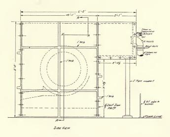
Fig. 2. A Pipe Welding Furnace operated with one burner and used for welding a flange on 20 in. pipe, for van-stoning, etc.
