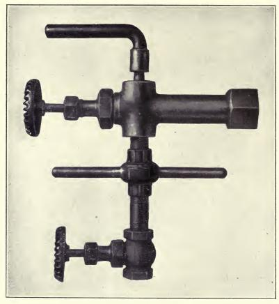
Fig. 3. Mechanical Burner.
