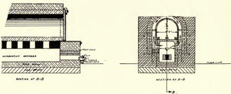
Muffle Furnace for Baking Enamel, Annealing, etc.
