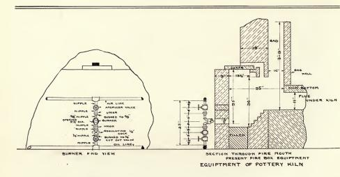
Two ways of equipping a pottery kiln, the type of construction shown in the upper views being the most modern.
