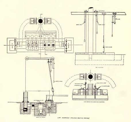
Fig. 2. A Modern six pot brass melting furnace.
