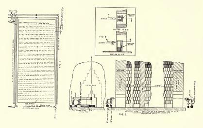
Fig. 1. An ordinary brick kiln, having 40 eyes, the capacity being 500,000 brick.
