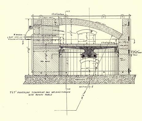
7 ft. x 7 ft. Annealing Furnace with Rotary Table.
