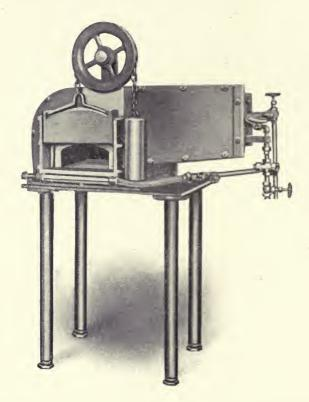
A small furnace which is used for a wide range of work in small shops. For instance, in many plants one of these little furnaces is used for forging, rivet heating, annealing, hardening dies, dressing high speed steel tools, and by placing a muffle in the charging space it is used as a muffle annealing and tempering furnace. It heats rivets uniformly and on 2½ gallons of oil per hour is equal to four coal forges, the maximum capacity being eight thousand ¾-in. x 3-in. rivets per day (ten hours).
