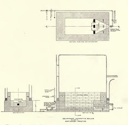
Fig. 4. Locomotive Boiler equipped for Stationary Service.
