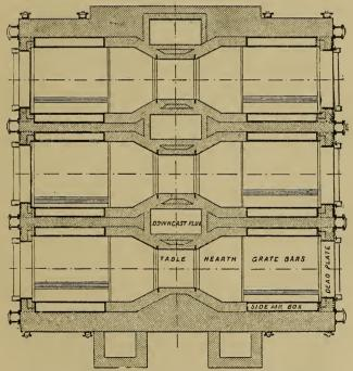
FIG. 53.—Plan at Grate Bar Level; Horsfall Destructor.
