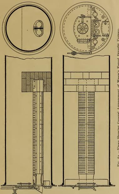
FIG. 6A.-Views Showing General Arrangement of Mason's Forced Draught Furnace.
