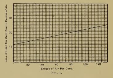
Some idea of the loss of heat through excess of air may be gathered from the accompanying diagram (Fig. 1).
