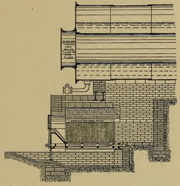
FIG. 14.—Longitudinal Section of Murphy Furnace as applied to a Lancashire Boiler.
