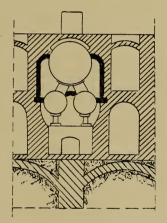
FIG. 32,-Transverse Section of Boiler Setting.
