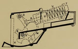
FIG. 23.-Showing Action of Sprinkling Shovel ; Bennis' Stoker.
