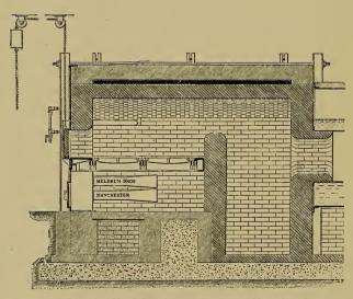
FIG. 43.—Longitudinal Section of Furnace, Showing Steam Jet Blowers; Meldrum's Destructor.
