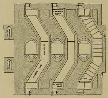
FIG. 55.—Plan at Level of Cross Flues; Horsfall Destructor.
