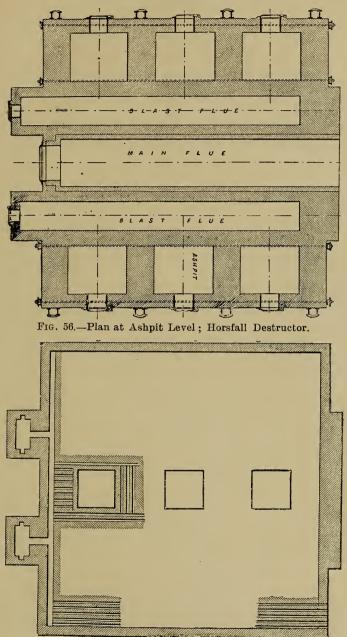
FIG. 57.-Plan Showing Air Passages ; Horsfall Destructor.
