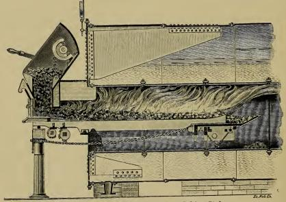
FIG. 30.-Longitudinal Section; Cass Coking Stoker.
