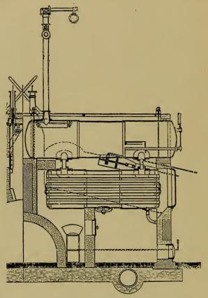
FIG. 59.-Section through one of the two Boilers.
