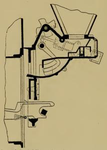
FIG. 28.—Section of Sprinkling Shovel Arrangement; Ransome and Rapier's Stoker.
