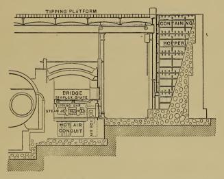
FIG. 37.—Section of Refuse Hopper, Grate, and Tipping Platform ; Meldrum's Refuse Destructor.
