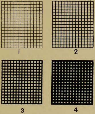
FIG. 31.-Ringelmann Smoke Test.
