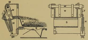
FIG. 20.-Showing Action of Sprinkling Shovel ; Proctor's Stoker.
