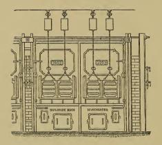
FIG. 42.—Furnace Doors; Meldrum's Destructor.
