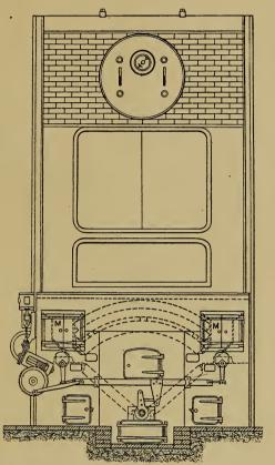
FIG. 12.—Front Elevation of Murphy Furnace as applied to a Water-tube Boiler.
