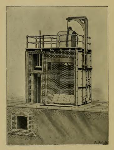
FIG. 44.—VIEW SHOWING INTERIOR CONSTRUCTION OF MASON'S SINGLE CELL REFUSE GASIFIER.
