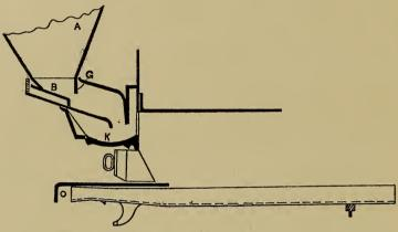
FIG. 21.—Longitudinal Section of Feeding Arrangement; Bennis' Sprinkling Stoker.
