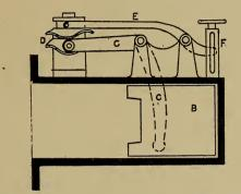
FIG. 22.—Sectional Plan of Feeding Arrangement; Bennis' Sprinkling Stoker.
