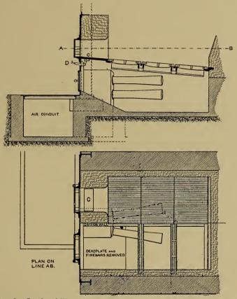
FIG. 6.—Sectional Elevation and Sectional Plan of Meldrum's Silent Blower.
