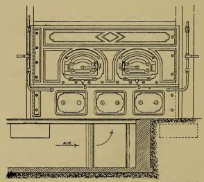
FIG. 5.—Front View of Meldrum's Silent Blower, as Applied to Water-tube Boiler.
