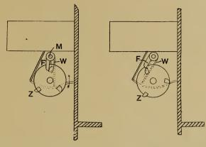
FIG. 19.—Tappet Cam Arrangement; Proctor's Sprinkling Stoker.
