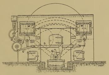
FIG. 10.—Front Elevation of Murphy Furnace as applied to a Lancashire Boiler.
