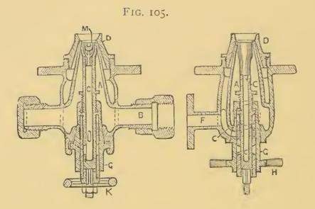
orifices O and the hollow spindle C into the circular opening M. In other respects the sprinklers remained unaltered, as the results attained with them were stated to have been highly satisfactory, and as much as 882 lbs. of oil were said to have been burnt per hour without any smoke being given off.
