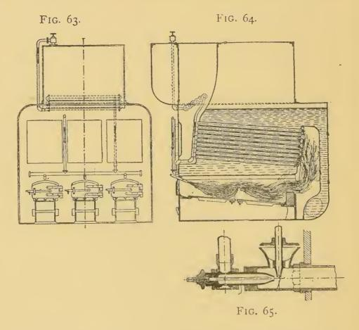
Lambeth in 1866 fitted to a Cornish boiler. The oil petroleum or tar oil—entered the sprinkler from a vertical pipe through an opening which was about 12 inches in diameter : through this opening it flowed continuously from a
