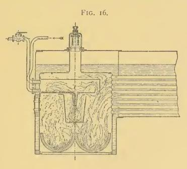
in 1862, and intended for locomotives and marine engines, represents the transition from hearth furnaces to gas furnaces. As shown at Fig. 16, the oil enters a reservoir in a tank in the furnace, and flows on to the fire-plate, which has been previously heated by a coal or wood fire. The lighter oils
