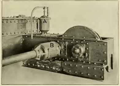
FIG. 13. SOME SAFETY FEATURES OF A TRAVELING CRANE. (This is a nearer view of some of the safeguards shown in Fig. 12. A is the track sander which is operated by a rope or cable attached to the lever and extended to the craneman's cage; B shows more clearly the drive-shaft coupling. The shaft inclosure also appears more plainly.)
