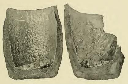
FIG. 7. A CRUCIBLE WHICH BROKE AFTER BEING RUN ONLY TWO HEATS.
