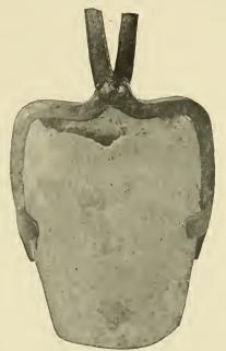
FIG. 10. TONGS PROPERLY APPLIED TO A CRUCIBLE, FOR REMOVING IT FROM A STATIONARY FURNACE.
