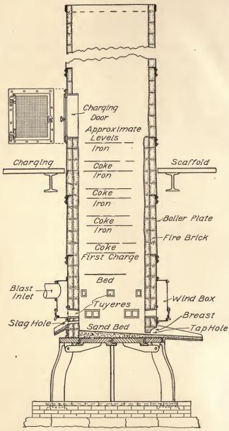
Fig. 98. Section Through Cupola Furnace.
