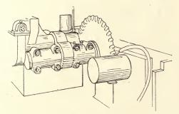
Fig. 124. Cutting off Riser.
