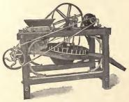
Fig. 132. Magnetic Scparator.
