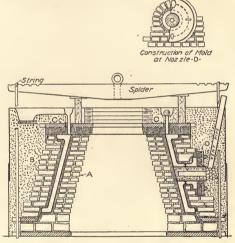
Fig. 96. Complete Typical Loam Mold.
