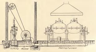
Flg. 136. Oil Furnace-General Elevation.
