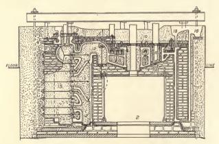
Fig. 97. Loam Mold for Marine Cylinder.
