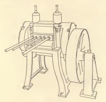
Fig. 115. Core Rod Straighteners.
