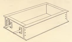
Fig. 118. Small Flask for Steel Molds.
