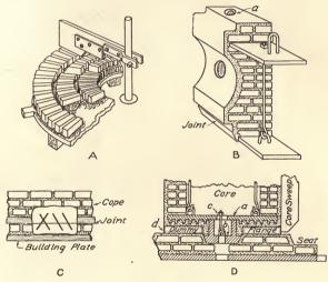
Fig. 94. Laying up Loam Work.
