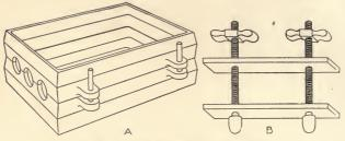
Fig. 125. (A) Flask for Brass.-(B) Screw Clamp.
