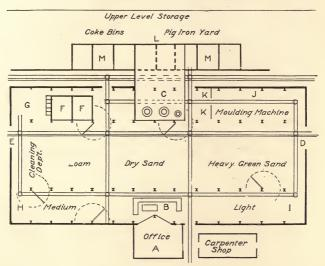
Fig. 137. Typical Plan of Foundry.
