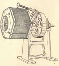
Fig. 107. Rotary Sieve.
