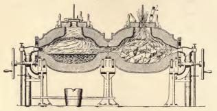
Fig. 135. Section Through Oil Furnace.
