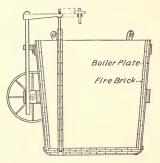
Fig. 122. Section Through Steel Ladle.
