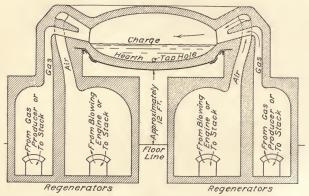
Fig. 120. Section Through Open Hearth Furnace with Regenerators.
