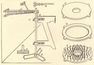
Fig. 93. Rig for Loam Work.
