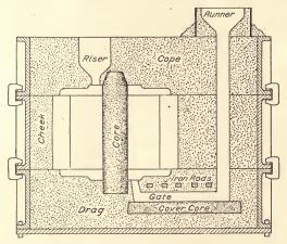
Fig. 119. Section Through Steel Mold.
