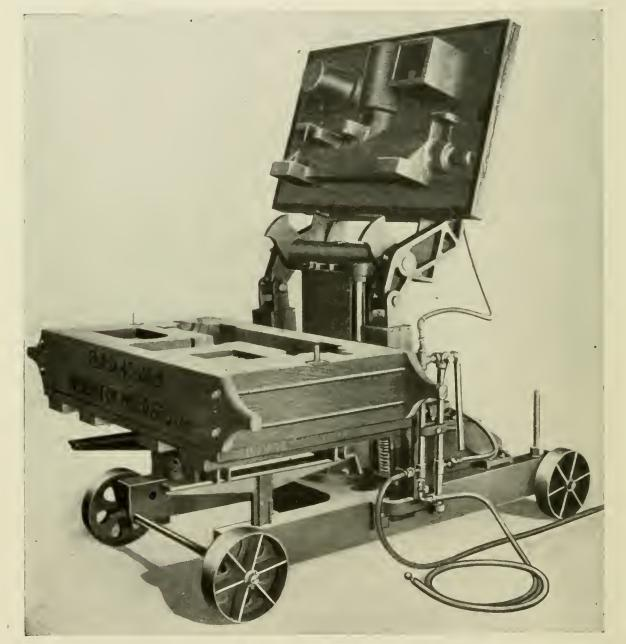
FIG. 208.—POWER ROLL-OVER AND POWER DRAFT MOLDING MACHINE.
