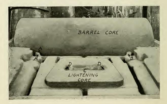
FIG. 106.—THE LIGHTENING AND BARREL CORES IN POSITION.
