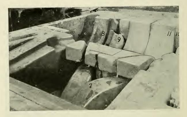
FIG. 119.—CHEEK PART OF THE MOLD, SHOWING Y-SHAPED EXHAUST CORE AT 7.
