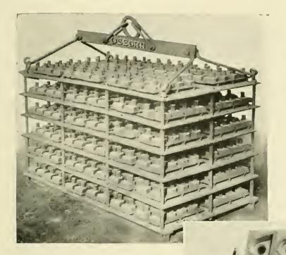
FIG. 167.—CARRIER USED FOR DISTRIBUTING CORES TO MOLDERS. BY CRANE OR MONORAIL.
