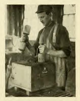
FIG. 4.—-BUTT-RAMMING THE SURFACE OF THE MOLD.
