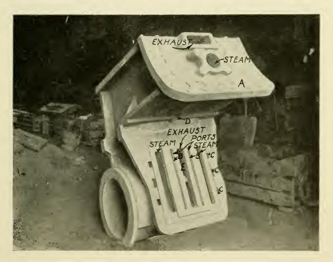
FIG. 99.-CYLINDER SHOWING STEAM ENTRANCE AND EXHAUST PORTS.
