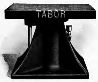
Fig. 91. A Small Plain Jolt Machine of Simple Construction.
