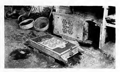
Fig. 162. Wood Forms Are Used to Shape the Ends of the Plate and Form the Pin Ears.
