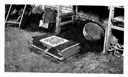
Fig. 157. The Gate of Patterns is Placed on the Match and an Extra Length of Green Sand Built On.
