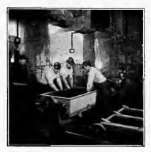
Fig. 81. Jolting the Drag Half of the Mould.
