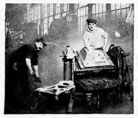
Fig. 30. Showing Clearly the Method of Pattern Mounting Employed.
