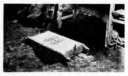
Fig. 159. The Hard Sand Match is Removed, Leaving the Pattern Bedded in the New Drag Half.
