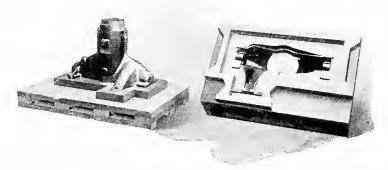
Fig. 137. A Wood Pattern on a Wood Plate with the Core Box on the Right.
