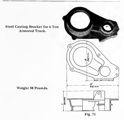
Production based on making both the cope and the drag half of mould on the same machine.
