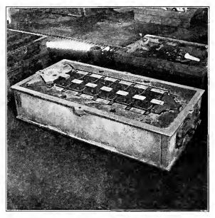
Fig. 84. Drag Half of Manual with Comes Sat
