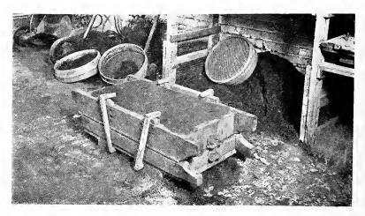
Fig. 164. The Pattern Having Been Drawn, the Mould is Closed and Clamped.
