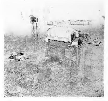
Fig. 214. Foundry Floor View of 42-inch Electrically Operated Roll Over Jolt-Moulding Machine, Showing Foundations in Phantom.
