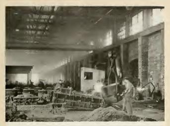
POURING STEEL INTO MOLDS AMERICAN CLAY MACHINERY COMPANY, BUCYRUS, OHIO
