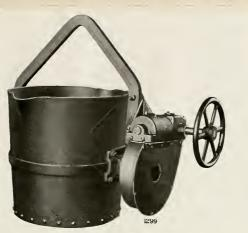
CRANE LADLE WITH ENCLOSED WORM GEARING
