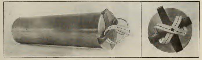
CARTRIDGE CASE WITH DRAWING CLIP ATTACHED.
