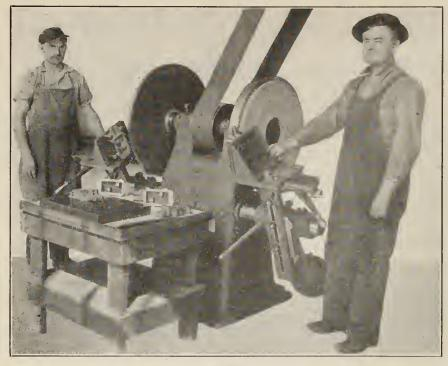
FIG. 3. GRINDING SMALL MALLEABLE IRON CASTINGS.
