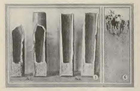
Fig. 6. Etching on axis line to determine amount of segregation. Fig. 8. Shell for gings from blanks (1) and (2) of Fig. 7, split open for inspection.
