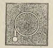
FIG. 1. GATING TO PRODUCE A SWIRLING MOTION.
