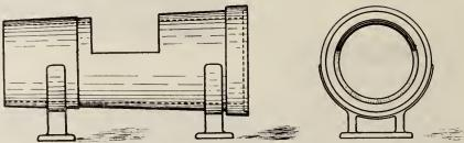
FIG. 20. JIG FOR TESTING TAPER AND OUTSIDE DIAMETER OF BACK ENDS.
