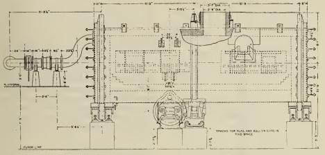
BASIC COPPER CONVERTER, PEIRCE-SMITH TYPE, MOND NICKEL CO VERTICAL LONGITUDINAL SECTION (A.C. CO.).
