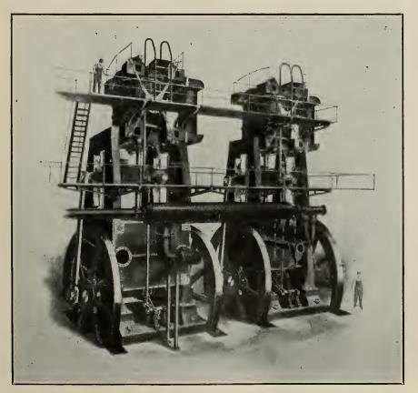
DISCONNECTED COMPOUND LONG CROSSHEAD BLOWING ENGINE.
