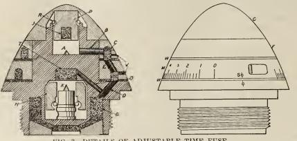
FIG. 3. DETAILS OF ADJUSTABLE TIME FUSE.
