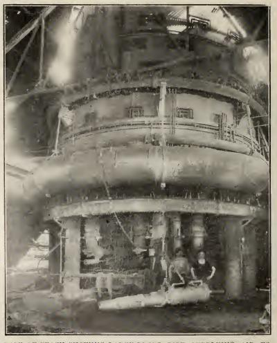
3ASE OF STACK SHOWING LARGE BLAST PIPE SUPPLYING AIR TO THE TUYERES. STEAM OPERATED MUD GUN IN FOREGROUND USED FOR PLUGGING TAP HOLE BEHIND THE MUZZLE.
