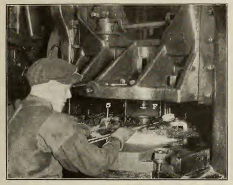
FORGING SOCKETS FROM BRASS SLUGS.
