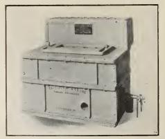
PREHEATED LEAD BATH FURNACE FOR SHELLS.
