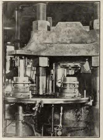
FIG. 15. HEADING 18-PDR. SHRAPNEL SHELL CARTRIDGE CASES ON AN 800-TON HDRAULIC PRESS. Note at the left foreground the small hydraulic ram which forces the cartridge case out of the dies and also the little jaws which hold it up from the dies as they return to their normal position.
