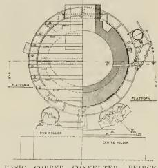
BASIC COPPER CONVERTER, PEIRCE-SMITH TYPE, MOND NICKEL CO., TRANS-VERSE SECTION THROUGH WIND BOX AND TIYERE ON RING NEAREST THE TILTING MECHANISM (A.C. CO.).
