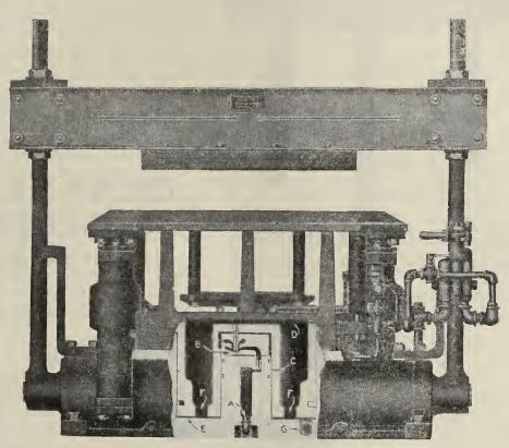
A-Air for Jolt Ramming. B-Automatic Single-piece Valve for Jolt Ramming. C-Exhaust from Jolt Rammer. D-Open joint between plunger and ramming head of machine through which exhaust escapes. E-4/" leather sheet serving as impact surface during jolting and valve closing surge ports FF during squeezing.
