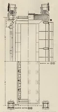
COPPER BLAST FURNACE, 1912, MOND NICKEL CO. HORIZONTAL TRANSVERSE QUARTER SECTIONS (A. C. CO.).
