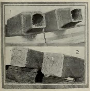
Fig. 1. 18-in, ingots of about 2% tons made by the "Hadfield" process. Fig. 2. 18-in, ingots of about 2½ tons. A-Unsound ingot. B-Piped ingot.
