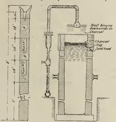
Fig. 7. Sketch showing upper portion of ingot forged and drawn out into a bar 434 in. diar. and about 8 ft. long. Fig. 9. Apparatus employed in producing sound ingots.
