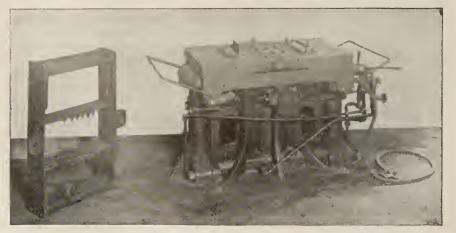
JOLT STRIPPING PLATE MACHINE READY TO RECEIVE FLASK.
