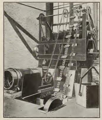
FIG. 1. MIXING, ROLLING AND BONDING MACHINE.
