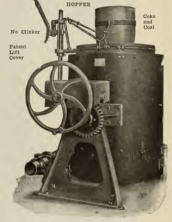
Furnace in Belting Position, Hopper Feed, Shaker Grates.
