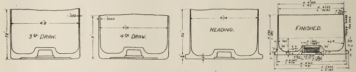
FIG. 23. SERIES OF OPERATIONS THROUGH WHICH THE 4.5 HOWITZER CARTRIDGE CASE PASSES IN THE PROCESS OF MANUFACTURE.
