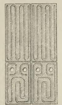
SECTION SHOWING ARRANGEMENT OF OF COOLING PIPES IN CAST IRON FURNACE JACKETS.
