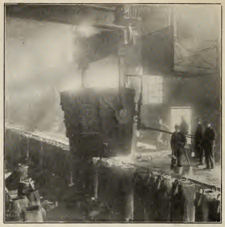
"TEEMING" THE MOLTEN STEEL INTO INGOT MOULDS.
