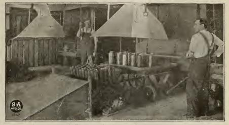
1. CARTRIDGE CASES BEING PICKED OFF PAN FROM ANNEALING FURNACE AND LOADED INTO WIRE BASKET ON CONVEYOR.
