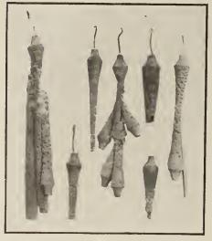
WELDED-UP SCRAP NICKEL ANODES.
