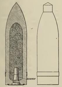
FIG. 1. SIMPLEST FORM OF EXPLOSIVE PROJECTILES.
