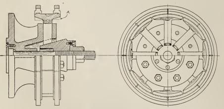
FIG. 4. IMPROVED DESIGN OF EXPANDING CHUCK.
