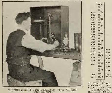
TESTING SHELLS FOR HARDNESS WITH "SHORE" SCLEROSCOPE.
