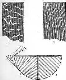
Figure 3. The end of log and how to cut so as to produce a desirable figure, as per cut No. 1. Letter A represents the first position of quarter on Head-block; B, second; C, third. The waste indicated by the wedge boards, (4 in number) as per cut No. 3, should be cut into half-inch boards, which are not objectionable.
