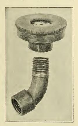
Fig. 12.—Large eddy-chamber or whirlpool-disk type of nozzle and elbow or crook. (Quaintance and Siegler.)
