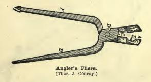
nosed pliers; B, knife for splitting shot; C, fine wire cutter; D, strong wire cutter; E, screw-driver; F, reamer. They weigh only four ounces, and are made of the best steel and in the best manner, and will be found thoroughly reliable. The cut is one half the size of the pliers. With this tool, a bit of string and a piece of wire, a broken rod or a disabled reel may be quickly remedied or repaired. It should be carried in every angler's pocket.
