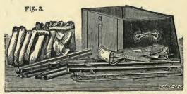
The above is a view of the boat in its compact or portable form, showing boat folded, bottom-board, camp-stools, gunwale, stretcher and packing-chest; oars and paddles are jointed, and pack in chest with boat.
