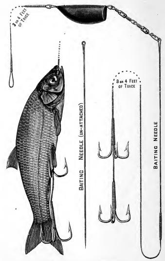
FIG. 2.—CENTRAL-LINK 2-TRIANGLE FLIGHT WITH TRACE (4½-inch bait). Showing also Baiting-needle detached from Trace. (Baiting-needle, Regd. No. 416122.)
