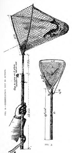
only by balance. By a sharp forward and then backward jerk of the net, which he now holds in his right hand, the length of the handle is doubled, and the total length of the net extended to four feet ten inches, of which three feet ten inches are represented by the handle and one foot by the net.
