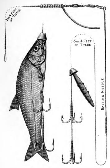
FIG. 1.—CENTRAL-LINK FLIGHT, 2 TRIANGLES (with 4½-inch bait), 'SWIVEL-COMPELLER,' AND TRACE-BAITING NEEDLE ATTACHED,
