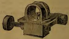
Fig. 9-Front sight, showing spirit level.
