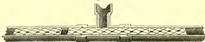
COTTAM'S IRON GUTTERING FOR CLOSED SURFACE STABLE-DRAINS.
