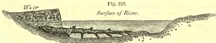
MISUSE OF A TREE IN THE PROTECTION OF RIVER-BANKS.
