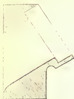
DOULTON'S PATENT JUNCTION BLOCK FOR DRAINS.
