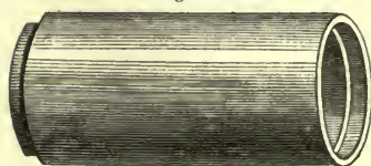
CLAYTON'S CORED-JOINT FOR DRAIN-TUBES.
