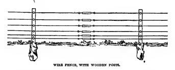
"The accompanying cut exhibits the natural size of the wires most commonly used for farm fences, and shows the manner in which they
