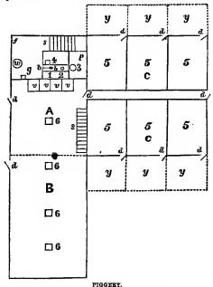
A, A, front; C, C, rear for pens; 5, 5, pens with alley between;  $\sigma$ ,  $\sigma$ ,  $\sigma$ ,  $\sigma$ , vats on level with pens; 1, safety valve; 2, steam pipe; 8, supply barrel to boiler;  $\delta$ , boiler; f, furnace;  $\rho$ , platform partly over boiler; 4. chimney;  $\delta$ , drain;  $\omega$ , water-clatern;  $\sigma$ , door to cellar; s, s, stairs;  $\tilde{\sigma}$ , d, doors; 6, 6, scuttles to cellar; v, y, yards to pens.
