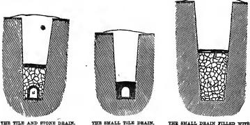
HE SMALL DRAIN FILLED WITH SMALL BROKEN STONES.
