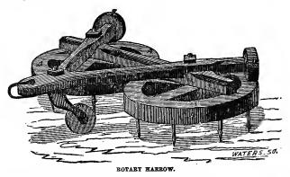
The accompanying engraving represents a harrow recently patented by Samuel J. Orange, of Graysville, Ill. It involves the rotary principle, the rotation being produced by the pressure of the rollers g g upon the wheels A A. It has the important advantage, that while it secures the rotation of the wheels, it at the same time avoids side draught.
