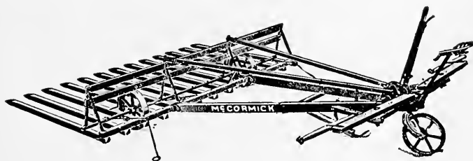
FIG. 133—A THREE-WHEEL SWEEP RAKE. THE DRIVER IS AIDED IN LIFTING THE LOADED TEETH BY THE PULL OF THE HORSES
