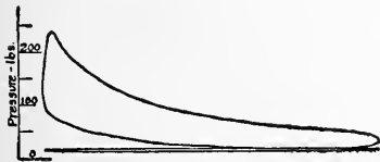
FIG. 15—AN ACTUAL INDICATOR DIAGRAM OBTAINED FROM A GAS ENGINE, WITH THE SCALE OF THE SPRING APPENDED
