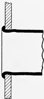
FIG. 240—FLUE EXPANDED WITH PROSSER EXPANDER
