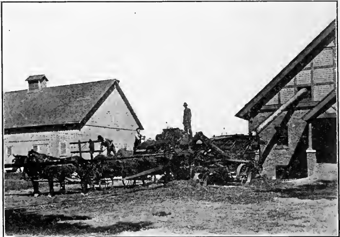
FIG. 154—A THRESHING MACHINE IN OPERATION. THE GRAIN IS SUPPLIED TO THE MACHINE FROM ONE SIDE IN ORDER TO OBTAIN A BETTER VIEW OF THE MACHINE
