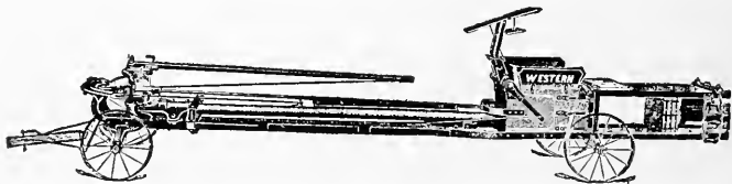
FIG. 143—A FULL-CIRCLE HORSE HAY PRESS ON TRUCKS FOR TRANSPORTATION
