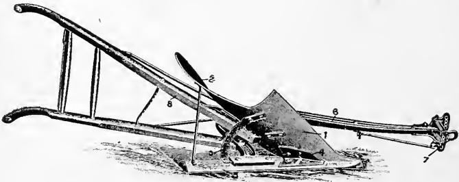
FIG. 34—AN UNDER VIEW OF THE MODERN STEEL PLOW, SHOWING ITS CONSTRUCTION
