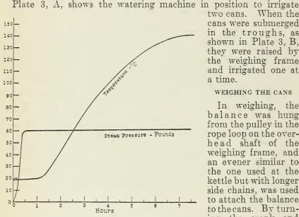
16.6.—Diagrammatic curves of the steam pressure in the kettle and the temperature in the interior of a can of soil in a represent-ative sterilization. In reading the steam-pressure curve the axis of ordinates indicates pounds; in reading the temperature curve it indicates degrees centigrade; and the axis of abscissas indicates time in hours for both curves FIG 6-
