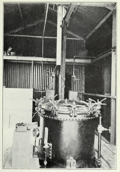
KETTLE FOR STERILIZING SOIL CANS, WITH ATTACHMENTS AND OTHER APPARATUS
