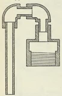
FIG. 2.—Cross section of the vent cap. It consists of a 34-inch to 14-inch reducer, into which fit successively two 14-inch elbows and a 14-inch pipe 3 inches long and open at the end. The elbows and upper two-thirds of the 14-inch pipe are closely packed with asbestos wool
