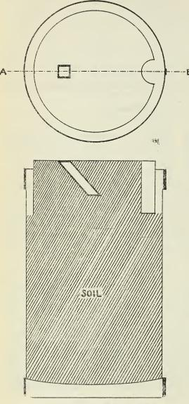
F IG. 5.—Diagrammatic representation of a top view of a filled soil can, showing the water shield and wooden block in place; also a vertical cross section of the can on the line A-B
