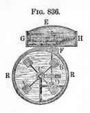
of the tachometer in a pipe. The vane-wheel in this case also puts a shaft D E in rotation by means of an endless screw; the former passes out of the pipe R R, in which the water to be measured flows, through a stuffing-box F into the case G H of the counting apparatus, the arrangement of which may be very varied.
