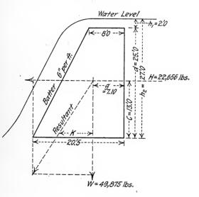
Horizontal Pressure  $H = d \times \frac{1}{2} (h_2 + h_1) \times 62.5 = 22\ 656\ 625$  lbs. Distance to Center Pressure,
