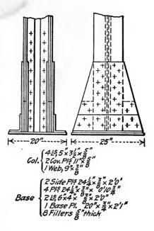
Assume 15 000 lb. per sq. in. bearing on rivets. 7 500 "" " " shear on rivets. 800 " " " " bearing on granite.  $\frac{400\ 000}{8\ 00} = 500 \text{ sq. in., base plate.}$
