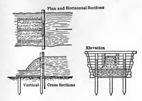
(b) Where there is no dam, a special weir may be constructed over the stream and the discharge obtained; or, the velocity gauged, the cross-section measured and the discharge computed by the formula Q = A v, or the Chezy-Kutter formula (see Q. 93), may be used, giving appropriate values to the constants s, n, and r as determined by measurements and observations.
