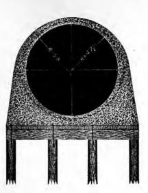
164. Explain the method of designing a masonry arch viaduct to carry an aqueduct.
