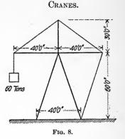
1. Determine the stresses in the members of this crane (Fig. 8), both analytically and graphically.
