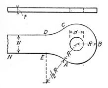
Let w = width of bar in inches. Then  $t = \frac{1}{4} w$  to  $\frac{1}{6} w$  (thickness of bar). d = 0.75 w to w = diameter of pin.
