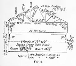
Allow 10 000 lb. per sq. in. shearing value on rivets. " 20 000 " " " " bearing value on rivets. " 250 " " " " pressure on bed plates.
