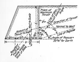
80. What should be the thickness at the top and base of retaining wall 15 ft. high, built to retain ordinary earth? Show a sketch of the wall, and how it should be founded.
