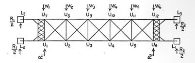
The above is a plan of the upper lateral and the portal bracing. The upper lateral system is calculated as a truss with panel loadings equal to the wind pressure per panel, the ends of the truss being at  $U_1$  and  $U_6$ .
