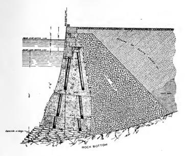
183. Make a sketch of the typical section of bulkhead in use at present where the bottom is good and depth moderate.
