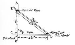
Let A B represent the line and C the point on it at which the offset is desired. Lay off 3 ft. from C, giving a point E. One man then holds the zero of tape at E and the 9-ft. mark at C. The tape is then pulled taut with a pencil held on the 5-ft. mark, which gives a point, D, on the offset line. Equi-multiples of 3, 4, 5, such as 6, 8 and 10; 12, 16 and 20, etc., may be used. The longer the distances used the greater the accuracy with which the offset may be laid off.
