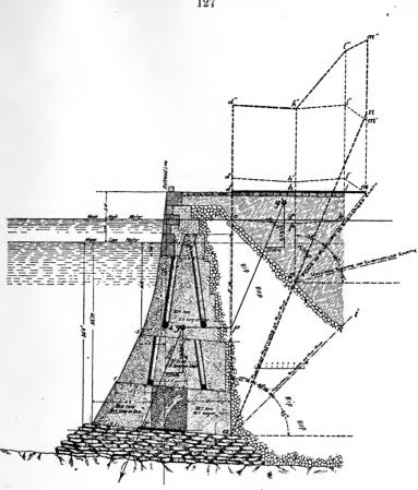
The forces acting against stability are: 1. The weight of the submerged rip rap..... 752. The weight of the submerged earth filling.... 703. The weight of the earth filling not submerged 110 4. The weight of the rip rap not submerged.... 110 5. Surcharge and liveload..... 1000 lb. per sa. ft.
