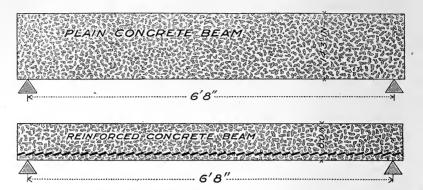
The fundamental principle of design may be stated as follows: In any structural member, mortar or concrete, reinforced by metal, is capable of sustaining very much greater elongations than when not reinforced and still effectually contribute to the resistance of the member.
