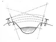
Let A and B be two bench marks, one on each side of river. With level at C determine difference in elevation between A and B. Do the same with level at D, making  $A \ C = B \ D$ . Let E' and E'' be the absolute elevations of A and B, then
