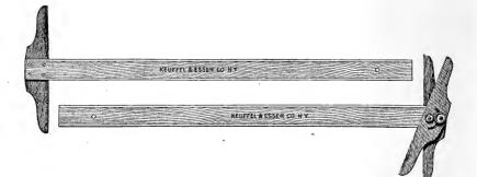
The "T" square is used to draw straight lines on the board, parallel to each other and perpendicular to the sides of the board. The head is placed firmly against the left-hand edge of the board, the upper edge of the blade is placed at the point through which it is desired to draw the line; the latter which is then drawn by passing the pencil or pen along the edge of the blade.
