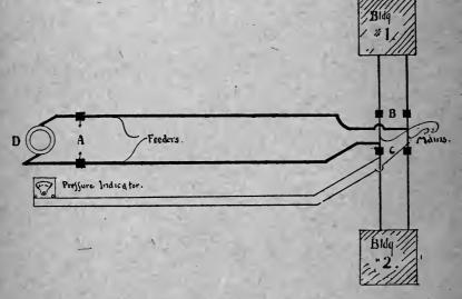
FIGURE 19.—PLAN OF CURRENT DISTRIBUTION SHOWING FEEDERS, MAINS AND PRESSURE WIRES.
