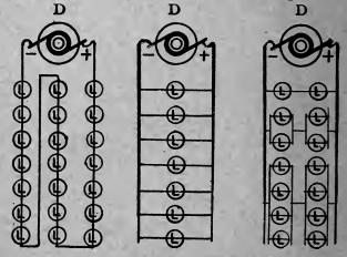
Series (a) Multiple or Parallel (b) Mulliple Series (c) FIGURE 2.—SYSTEMS OF CURRENT DISTRIBUTION.
