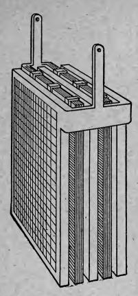
FIGURE 37.—STORAGE BATTERY PLATES. PASTED PLATE TYPE.
