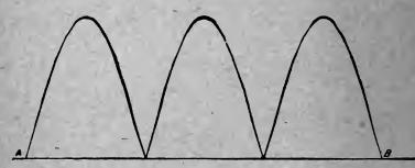
FIGURE 7.—PULSATING DIRECT CURRENT WAVE— SINGLE COIL ARMATURE.
