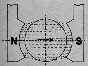
FIGURE 9.—FLOW OF MAGNETISM THROUGH A DRUM ARMATURE CORE. magnetism will take to the iron in completing their individual circuits, and so it has been found advisable to wind armature coils on an iron core, so that the largest possible number of lines of magnetism flowing from the poles of the field magnets, will flow through the iron armature cores, and in this way, the coils of the armature will cut a larger portion of the lines given out by the field magnets.
