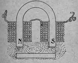
FIGURE 3.—ELECTRO-MAGNET AND ARMATURE SHOW-ING LINES OF MAGNETISM.
