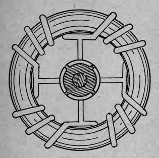
FIGURE 12.—GRAMME RING ARMATURE. FOUR COIL TYPE.
