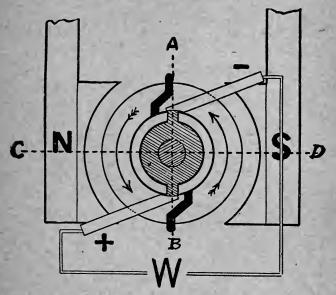
FIGURE 5.—SINGLE LOOP ARMATURE ON IRON CORE WITH COMMUTATOR AND BRUSHES.
