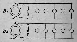
FIGURE 21 — TWO DYNAMOS SUPPLYING 5 LAMPS EACH, ON MULTIPLE SYSTEM.
