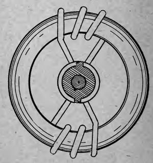
FIGURE 11.—RING ARMATURE.—TWO COILS IN MULTIPLE.
