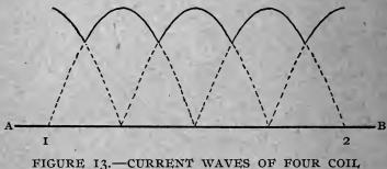
FIGURE 13.—CURRENT WAVES OF FOUR COIL RING ARMATURE.
