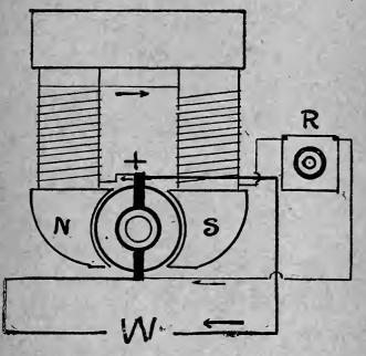
FIGURE 17.-SHUNT WOUND DYNAMO.
