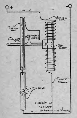
FIGURE 31.—CONNECTIONS OF CIRCUITS OF DIFFEREN-TIAL ARC LAMPS.—CLUTCH TYPE.
