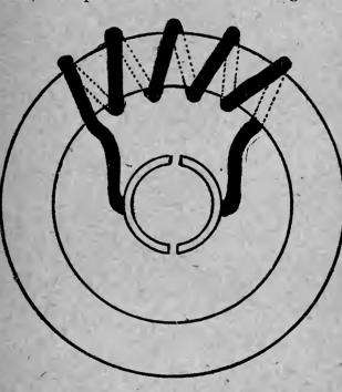
FIGURE 10.-RING ARMATURE OF ONE COIL.
