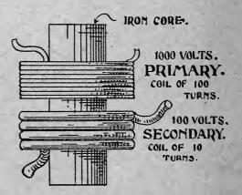
FIGURE 25.—IRON CORE WITH PRIMARY AND SECONDARY COILS.
