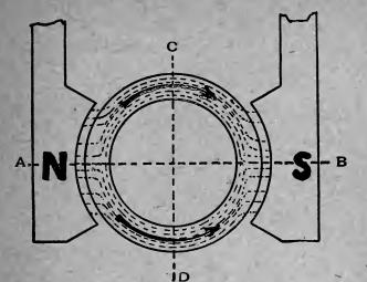
FIGURE 8.—FLOW OF MAGNETISM THROUGH A RING ARMATURE CORE.
