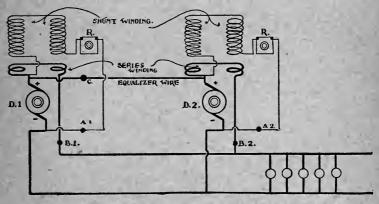
CONNECTIONS OF TWO COMPOUND DYNAMOS IN MULTIPLE,
