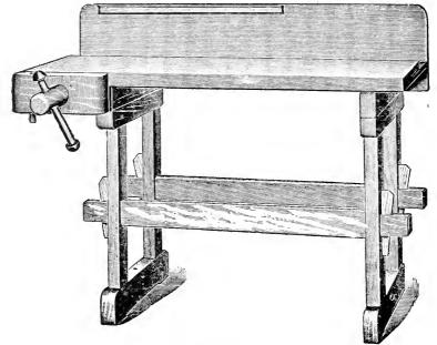
Fig 20. Wood Working Bench Keyed Mortise and Tenon
