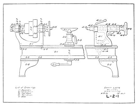
Fig. 33. Bench Lathe—Assembly.
