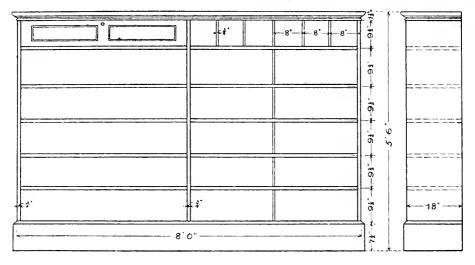
Fig. 25. Lockers for Wood Working Room.
