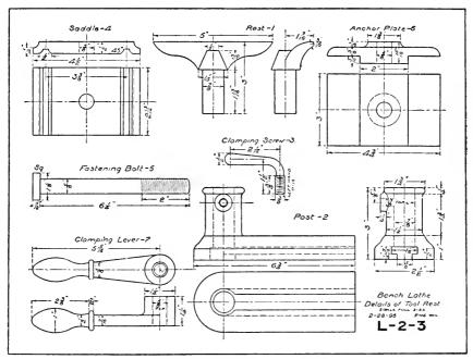
Fig. 35. Bench Lathe-Tool Rest.
