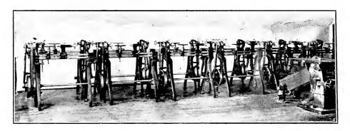
Fig. 32. Wood Turning Equipment Without Overhead Shafting.
