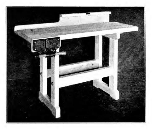
Fig. 19 Wood Working Bench. Draw Bolt Construction.
