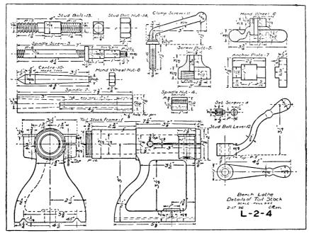
Fig. 36. Bench Lathe-Tail Stock.
