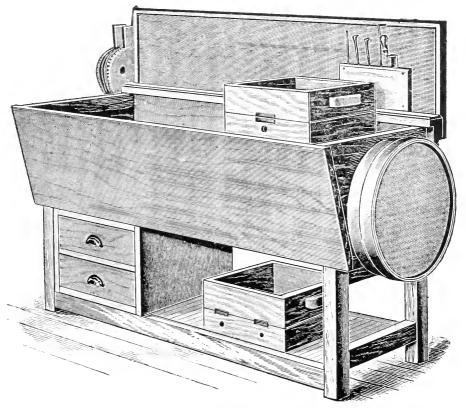
Fig. 41. Foundry Moulding Trough.
