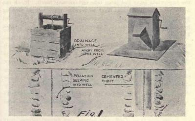
In the case of wells and springs, due to the filtering and purifying action of the soil, water from such sources is usually pure unless contaminated by some man-made cause, such as privies, cesspools or barn yards. See Fig. 1. For wells and springs, then, the problem is primarily one of protection.
