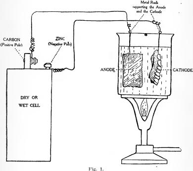
Scheme for arranging a simple electroplating outfit.
