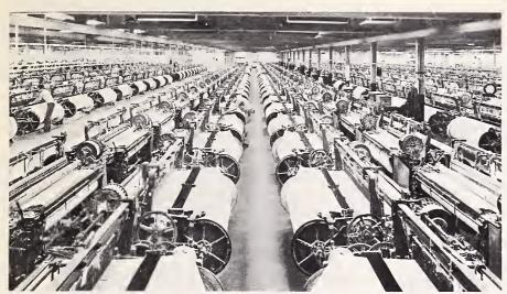
Figure 23 Weaving—The loom is used for weaving yarn into fabrics by interlacing two systems of threads at essentially right angles to each other. The lengthwise threads are called warp yarn and the crosswise ones are the filler or "welt" yarn.
