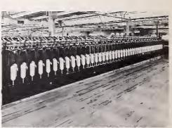
Figure 19 Roving—The roving process which follows drawing is designed to reduce the cotton strand to a progressively smaller diameter, give it a slight twist, and wind it onto bobbins.
