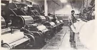
Figure 16 Picking—After bales of cotton have been opened and layers from each fed by turn into the opening machines which mixes, blends and cleans the fiber, the cotton is conveyed to the picker, which further opens and cleans the cotton and forms it into an even, flat sheet which is rolled into a lap about 18 inches in diameter and 45 inches wide.
