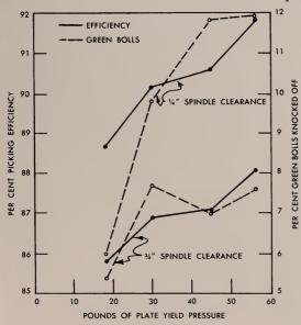
The picker efficiency was significantly affected by both the yield pressure and the spindle clearance. There was an increase of  $2\frac{1}{2}$  to 3 per cent in picker efficiency between the lowest and highest pressures. The  $\frac{1}{4}$  inch spindle clearance gave 3 to 4 per cent higher efficiency than the  $\frac{3}{4}$  inch clearance. The unharvested cotton was about equally divided between that left on the plants and that dropped on the ground.
