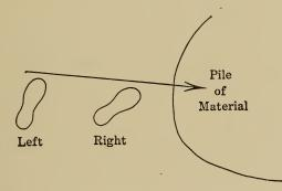
FIG. 2.—Position of feet for right-hand shoveler using long-handled shovel. Arrow shows direction of shovel.
