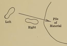
Fig. 1.—Position of feet for right-hand shoveler using a D-handle shovel. Arrow shows direction of shovel.
