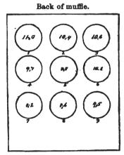
FIG. 3.—Position of cupels in muffle.
