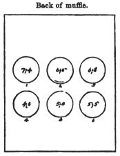
FIG. 4.—Position of cupels in muffle,
