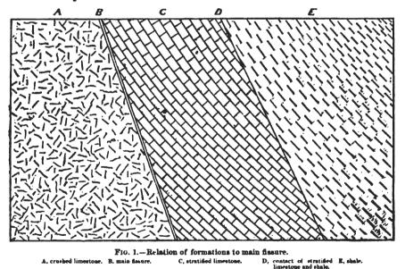
in the first north cross-cut 182 feet from the main drift. Between it and the shale the stratified limestone, which is here 30 feet wide, can be first definitely distinguished. This band of limestone, which increases in width as depth is attained, is always found on the hanging-wall side of the fissure,
