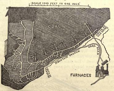
The original point of opening is seen to the left, while the tunnel from which the chief supply is now drawn is on the extreme right. The usual dip of the coal is from 30 to 35 degrees. This diagram was made by Col. Killebrew in 1877, and while it serve the design of showing how the coal has been mined, does not now truly exhibit the present interior shape of the mine. The arrows indicate the dip of the coal.
