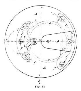
at Figs. 24 and 25. This model is supposed to have an escape wheel one-fifth the size of the 10" one we have been drawing. In the accompanying cuts are shown only the main plate and bridges
