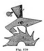
Fig. 168. At the moment of impact their extreme ends recoil or spring back from the shock of the escape teeth, but the resiliency of the metal is calculated to be strong enough to return them immediately to the contact studs e.e.
