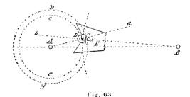
angular extent on the circle c, and if we make the passing hollow occupy eighteen degrees (which is one and a half the angular extent of the jewel pin) it will do nicely. But if we should extend the width of the passing hollow to twenty-four degrees it would do no harm, as the jewel pin would be well inside the horn of the fork before the guard pin could enter the passing hollow.
