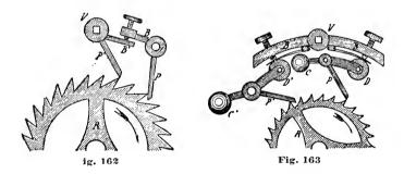
upon the pallet P, and the tooth b of the ratchet will encounter the pallet P'. This pallet, after suffering its recoil, will receive the impulse communicated by the tooth b. This escapement surely could not have given much satisfaction, for it offers no advantage over the others, besides it is of very difficult construction.
