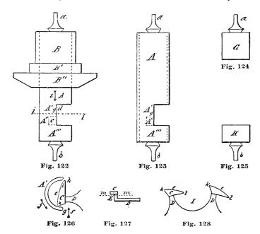
said cylinder must turn or revolve a little in the direction of the arrow j, and also that the next succeeding tooth of the escape wheel will engage the cylinder on the outside of the half shell, falling on the dead or neutral portion of said cylinder, to rest until the hair-spring causes the cylinder to turn in the opposite direction and permitting the tooth now resting on the outside of the cylinder to assume the position shown on the drawing.
