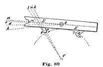
in the momentum of the balance has to actually turn the train backward and against the force of the mainspring. True, it is only through a very short arc, but the necessary force to effect this has to be discounted from the power stored in the balance from a former impulse. For this reason we should make the angular motion of unlocking as brief as possible. Grossmann, in his essay, endorses one and a half degrees as the proper lock.
