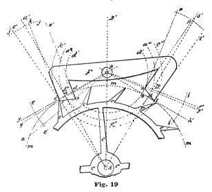
at s) does not have to be carried down on the arc d' as far to insure a continuous pallet action of ten degrees, as with the pallets with equidistant locking faces. Still, even here we have carried the angle s down about half a degree on the arc d', to secure a safe lock on the exit pallet.
