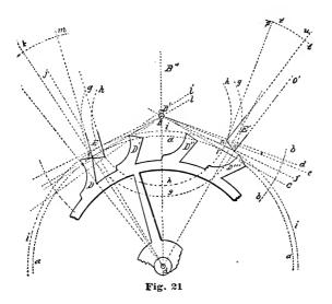
that the line A k is not at right angles to the line s l; and, consequently, the locking face of the entrance pallet E has not really the twelve-degree lock we are taught to believe it has.
