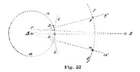
order we draw our jewel pin as shown at D. In drawing the jewel pin we proceed as at Fig. 56, except we let the line Ag', Fig. 57, assume the same relations to the jewel pin as AB in Fig. 56; that is, we delineate the jewel pin as if extending on the arc a six degrees on each side of the line Ag', Fig. 57.
