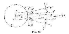
which, in case we employ a pitch circle of 5'' radius, would make the distance between A and B, Fig. 55, approximately  $7\frac{1}{2}''$ , which is a very fair scale for study drawings.
