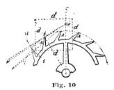
up to the present time, no remedy has been devised to overcome it. All the other escapements, including the chronometer, duplex and cylinder, are quite as wasteful of power, if not more so. It is usual to construct ratchet-tooth pallets so as to utilize but ten degrees of escape-wheel action; but we shall show that half a degree more can be
