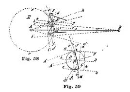
pin. This arc, carried across the jewel pin D, limits the length of the opposite prong of the fork. The outer face of the prong of the fork can be drawn as a line tangent to a circle drawn from A as a center through the angle n of the jewel pin. Such a circle or arc is shown at o, Figs. 58 and 59. There has been a good deal said as to whether the outer edge of the prong of a fork should be straight or curved.
