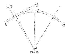
the center A so it would engage or rest on the locking face of the entrance pallet as shown at Fig. 84, then the draw of the locking angle would not be quite fifteen degrees; but it is evident no lock can take place until the angle a of the entrance pallet has passed inside the circle s. We would say here that we have added the letters s and t to the original drawings, as we have frequently to
