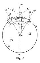
against a surface which coincides with the radial line pf, the action would be in the direction of the line fh and at right angles to pf. If we reason on the action of the tooth D, as it presses against a pallet placed at f, we see the action is neutral.
