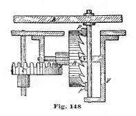
watches: B represents the regulator in the form of a circular balance, but not yet furnished with a spiral regulating spring; c is the last wheel of the train and called the *fourth wheel*, it being that number distant from the great wheel. As will be seen, the verge provided with its pallets is vertically placed,
