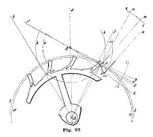
From the intersection of the line B e with the arc i we lay off two and a half degrees on said arc, and through the point so established we draw the line B g. The intersection of this line with the arc k we name the point z. With one leg of our dividers set at A we sweep the arc l so it passes through the point z. This last arc defines the addendum of the escape-wheel teeth. From the point r on the arc a we lay off three and a half degrees, and through the point so established draw the line A j.
