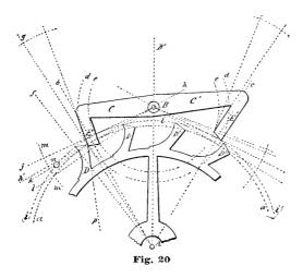
the dividers, and on the arc a a lay off the said two and a half degrees to the left of this intersection, and through the point so established draw the radial line A g. From B as a center we sweep the arc d d so it passes through the point of intersection of the arc a with the line A g.
