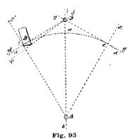
instance, the radius of the arc a is 5". After the drawing is in the condition shown at Fig. 93 we measure the distance on the line b between the points (centers) A B, and we thus by graphic means obtain a measure of the distance between A B. Now, by the use of trigonometry, we have the length of the line A f (radius of the arc a) and all the angles given, to find the length of f B, or A B, or both f B and A B. By adopting this policy we can verify the measurements
