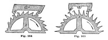
regulating the opening between the pallets. The counter-weight  $\mathcal{C}$  compels constant contact between the arms  $\mathcal{B}$   $\mathcal{B}'$ . The function is always the same, the recoil and the impulsion operate upon the two pallets simultaneously. This escapement enjoyed a certain degree of success, having been employed by a number of horologists who modified it in various ways.
