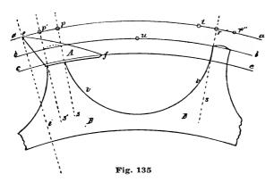
delineate an escapement in which the cylinder is correct but the teeth faulty; also change the thickness of the cylinder shell, so as to make the teeth too short. This sort of practice makes the pupil think and study and he will acquire a knowledge which will never
