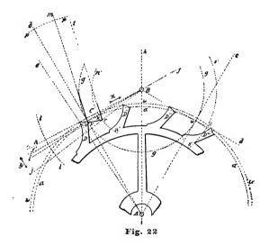
pallet staff B, with no tendency on the part of the pallet to turn on its axis B. Theoretically, the pallet with the locking face cut to coincide with the line A b would resist movement on the center B in either direction indicated by the double-headed arrow y.
