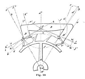
thirty degrees from the brass degree arc, and through the points thus established are drawn the radial lines a b' and a d'.
