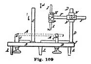
The seat a of the swing jaws C must hold the watch plate A exactly parallel with the bed plate B. In the cheap movement holders these seats (a) are apt to be of irregular heights, and must be corrected for our purpose. We will take it for granted that all the seats a are of precisely the same height, measured from B, and that a watch plate placed in the jaws C will be held exactly parallel with the said bed B. We must next provide two pillars,
