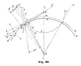
center of our pallet staff at B. At two and a half degrees from the point c we lay off two and a half degrees to the right of said point and establish the point n, and draw the radial line A n n', which establishes the extent of the arc of angular motion of the escape wheel utilized by the pallet arm.
