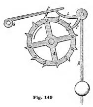
Here it will quickly be seen that regarded from the stand-point of regularity of motion, this arrangement can be productive of but meager results. Subjected as it is to the influence of the slightest variation in the motive power and of the least jar or shaking, a balance wheel escapement improvided with a regulator containing within itself a regulating force, could not possibly give forth anything else than an unsteady movement.
