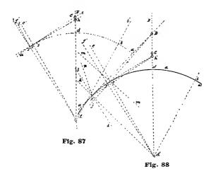
faces of the teeth. We will, for the present, accept the thickness of the arms as being equivalent to five degrees of angular extent of the pitch circle of the escape wheel.
