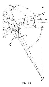
the escape wheel in its entire effort passes through eleven degrees of angular motion, while the pallets and fork move through ten degrees. The student will thus see we have arranged to give the train-power an advantage where it is most needed to overcome the opposing influence of the hairspring.
