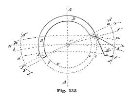
A little study of what would be required to get the best results after making such a drawing will aid the pupil in arriving at the peoper shape, especially when he remembers that the thickness of the cylinder shell of a twelve-line watch is only about five one-thousandths of an inch. But because the parts are small we should not shirk the problem of getting the most we possibly can out of a cylinder watch.
