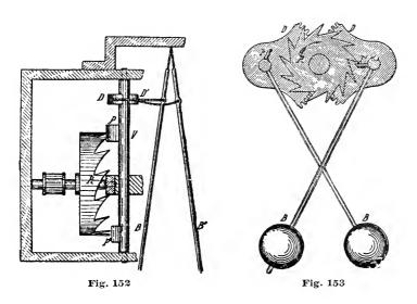
forked arm was not thought of, for the pendulum itself formed a part of the verge. A far-reaching step had been taken, but it soon became apparent that perfection was still a long way off. The crownwheel escapement forcibly incited the pendulum to wider oscillations; these oscillations not being as Galileo had believed, of unvaried durations, but they varied sensibly with the intensity of the motive power.
