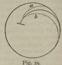
what is meant. If the full line represents the original form of curve, it would be altered in the direction of b to quicken the short, and in the direction of a to quicken the long arcs. To alter the shape of the overcoil the spring is held with a pair of tweezers with brass faces curved exactly to suit it, while the alteration is made with a similar pair. Alterations must be made very gradually, for if bent too much the spring is likely to be spoilt in bending it back.
