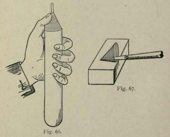
pointed peg charged with red stuff, the spring taking the form of a cone the while, as shown in Fig. 67.
