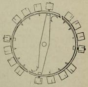
Fig. 24. Compensation Balance for Watches.
