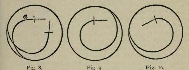
throwing the end inwards. This little bend is of the utmost importance, for it has the effect of quickening the short arcs. Pocket chronometer springs are made half the diameter of the balance, and from seven to ten turns.
