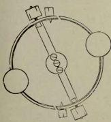
Fig. 23. Marine Chronometer Balance.
