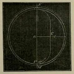
Fig. 12. to the left of the centre away from the centre, or by a combination of these operations. With left handed springs the correction would of course be in the reverse direction.
