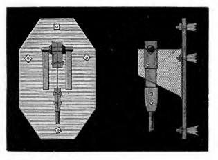
have shown the chops and spring and a side view of the cock and the plate belonging to it, and the *lewises* of the bolts. I have also given a front view of the form of plate which appears to me the best for obtaining steadiness with four bolts.
