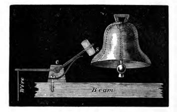
of the bell is so curved, that a tangent to it would make an angle of about  $35^{\circ}$  with a horizontal plane: and therefore the axis C of the hammer must be so placed that CS will form that angle with the horizon. As in house clocks the hammer is prevented from jarring on the bell by a spring as shown in the drawing.
