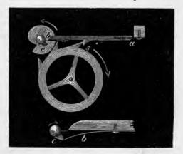
through a very small angle is set upon a small and stiffish spring at a instead of a pivot, which allows it to move just as a pendulum spring does a pendulum. The other end of H 3
