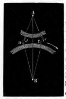
In this figure, D, C, represent two teeth of the driving wheel, and d, c, two corresponding teeth of the driven wheel. Now, although they are here represented as inclined to each other at the same angle in each case, yet any one must see at once that the friction between C and c, after the line of centres, is very much less than between D and d, before the line of centres : no degree of friction (short
