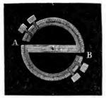
more than the inside steel ones, and so their ends, with the additional weight of the screws, bend inwards towards the centre of the balance, and its moment of inertia is diminished. The proper adjustment of these screws is, as may be supposed, a very delicate operation, and requires a great
