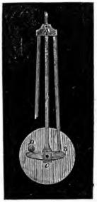
ratio of the long arm to the short arm of each lever is the same as that of the amount of expansion of the rod A B to that of the main rod, it is evident that the bob will be kept in the same place. Theoretically A may be anywhere, and A B may be either of iron or of brass; but the less expansion A B has the shorter must be the short arm of the lever, which is objectionable for several obvious reasons. A more serious objection to the pendulum altogether is
