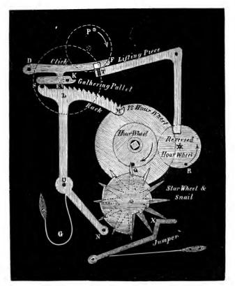
centre O, and having 13 or 14 ratchett shaped teeth on it. Another radius O N of this fragment of a wheel has a pin N set upon it; and on a wheel called the *star wheel*, which will be described presently and turns in 12 hours, there is fixed a graduated *snail* with 12 steps in it, such that when the hour hand points to 5 for instance the pin N can fall against the 5th step in the snail to such a depth that the rack can fall through the space of 5 of the teeth. The
