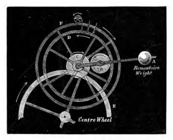
the internal teeth of D. Consequently, whenever the wheel D is driven by the train it will raise the right side of B, which will raise the lever and the weight; but the left side of B will nevertheless be always pressing downwards on C and tending to turn it the opposite way to D; and therefore a large wheel F fixed to the wheel C may be employed to drive the scape-wheel, which will then be driven merely by the remontoire weight and not by the clock train.
