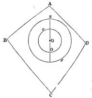
plane perpendicular to the axis of suspension is A B C D revolving round its centre of gravity G, and we make it revolve or oscillate about a new axis through S, and we want to know what is the length SO of the equivalent simple pendulum; it may be proved that  $SO = \frac{k_1^2 + SG^2}{SG}$  and  $\therefore GO = SO - SG = \frac{k_1^2}{SG}$ .
