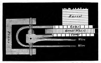
to be a strong stop (if cast on the frame all the better) for the *long* arm of the levers to strike against when the hammer falls, to take the shock off the striking pins, and, as far as possible, off the arbor. Such stops are often put to the short arm, and much too weak, and too near the arbor.
