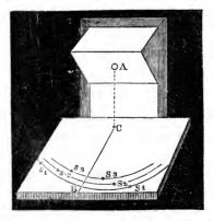
From A the hole in the plate drop a perpendicular A C upon the board, and make a mark at C. At a little after 11 o'clock on a fine day, observe where the image of the Sun falls on the board, and mark the place of its centre
