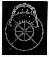
to be stopped by the short pallets containing only the dead part, which however is to have a small recoil in it. In that case the impulse might be given through a small angle near the middle of the vibration; and the pressure which causes the dead friction would be less
