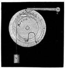
wheel and the barrel ratchett: this wheel has also ratchett teeth cut upon it, but turned the opposite way to the barrel ratchett, as shown at R, and the click R C belonging to it is a long arm turning on a pivot C in the clock-frame; and this second ratchett wheel is connected with the great wheel in any convenient way by a spring S S, having one end fixed on the ratchett wheel, and the other end pressing against a pin on the great wheel. The action is this: while the
