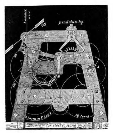
plate set upon a stud outside. The numbers of the teeth which I have inserted are of course arbitrary, and may be altered in the proper proportions.
