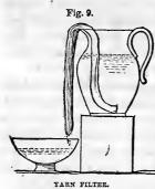
represented in fig. 9. A thick wick or skein of cotton or worsted thread is hung over the edge of a deep basin or jar; and the water follows the course of the threads, by what is called capillary attraction, leaving the impurities behind. The filtration, however, is not as complete as by other methods.
