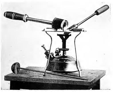
FIG. 28.-A kerosene stove which burns a gas flame for heating soldering tools.
