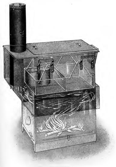
Fig. 57.—Showing construction of a hot-water canner. (Phillips & Buttorff, Nashville, Tenn.) soldered together, the solder will melt and the water will leak out, making the canner useless until it is mended.
