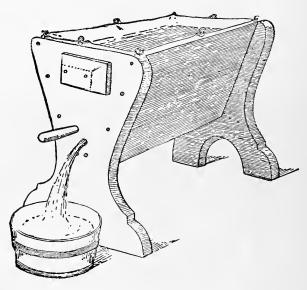
FIG. 72.-A homemade fruit-juice filter.
