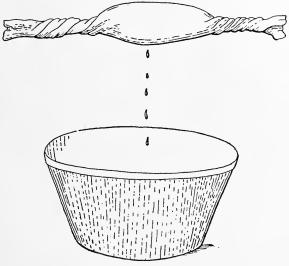
FIG. 68.-Cloth press being twisted.
