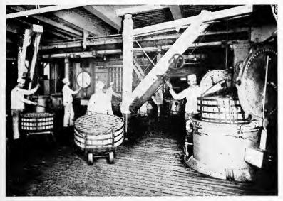
FIG. 66.—Commercial retorts where steam is piped in from the boiler. (Heinz Company.) TIME-TABLE FOR PROCESSING BY STEAM
