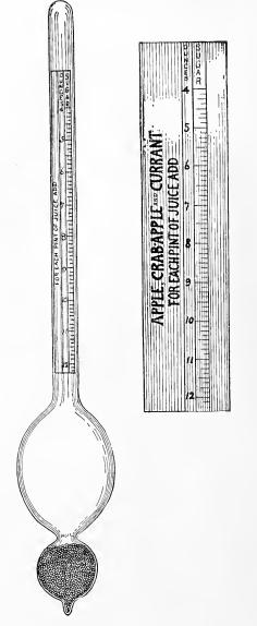
F16. 101.-Jellometer for testing fruit juices in jelly making.
