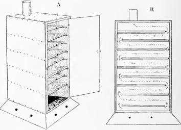
F1G. 120.—A. Homemade cook-stove drier. B. Sectional view showing the passage of the heated air.
