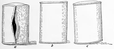
F1: 14.—(a) Can burst from pressure of gas generated; (b) a normal can; (c) a swell.
