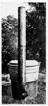
FIG. 56.—A homemade canner with brick fire-box and tub.
