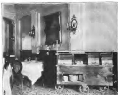
**ELECTRIC WAGON**, made of German silver and brass. Carries two meat platters, four vegetable compartments and one gravy. Plate warmer below and elevated service shelf above. Is about six by two feet, on heavy swivel rubber tired casters. Equipped with electric heat units, and with cord and plug to be connected to electric stations in kitchen and dining rooms.
