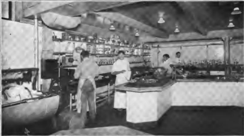
**SILVER WASHING AND CLEANING DEPARTMENT** (Davenport Hotel, Spokane): Tahara machine shown open at left, with silver in bath of shot and suds. Note the care in handling, in particular placing the wiped silver on mat. The Blakeslee rotary silver washing machine is located behind the soiled silver table at right. Note the sanitary enclosure of this department, all white tile wall with sanitary covered base.
